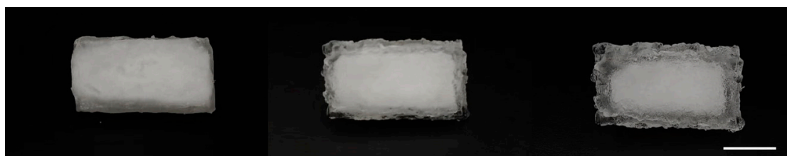
Figure 1. Photographs of PAM-LiCl before water capture (left), water uptake of 0.5 g/g (middle) and 1 g/g (right); Scale bar: 1 cm.
