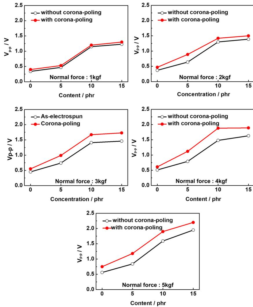
Figure 5.  $V_{p-p}$  values of sensors fabricated from PLA/BTNP nanofiber webs with and without corona-poling treatment as a function of the concentration of BTNPs and the normal force applied to the sensors.
