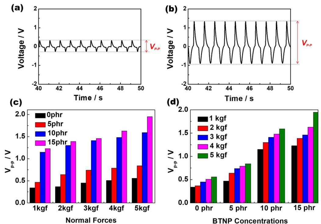
**Figure 3.** Typical profiles of piezoelectric voltages ( $V_{p-p}$ ) of the sensors fabricated from electrospun (a) PLA and (b) 15 phr BTNP-doped electrospun PLA nanofiber webs. (c) The dependence of  $V_{p-p}$  on BTNP content under different normal forces (pressure). (d) The dependence of  $V_{p-p}$  on normal forces under different BTNP concentrations.
