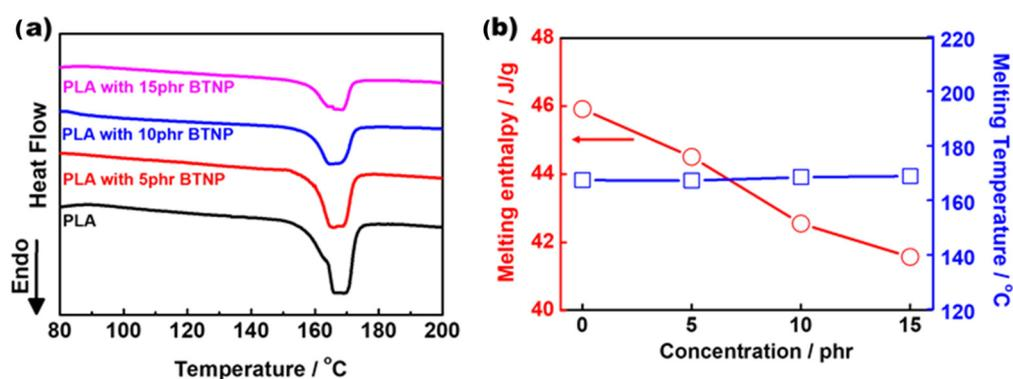
**Figure 4.** (a) DSC melting traces of electrospun PLA and electrospun PLA/BTNP nanofibers. (b) Melting enthalpies and temperatures of BTNP concentrations.
