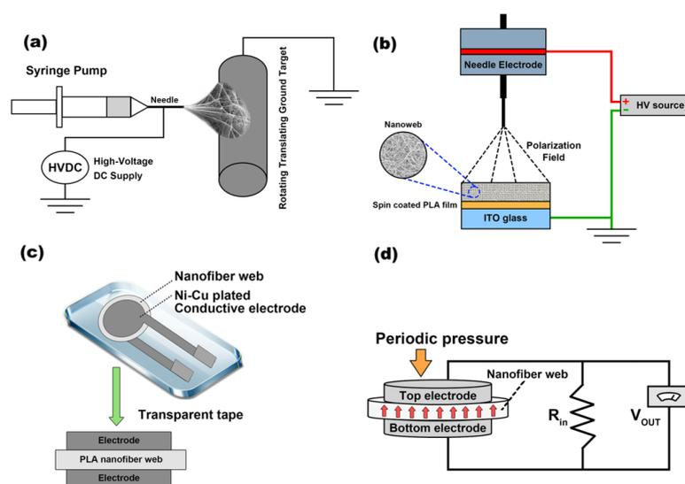
**Figure 1.** (a) Electrospinning experimental setup. (b) Corona-poling setup. (c) Sensor structure. (d) Custom-built dynamic pressure instrument.
