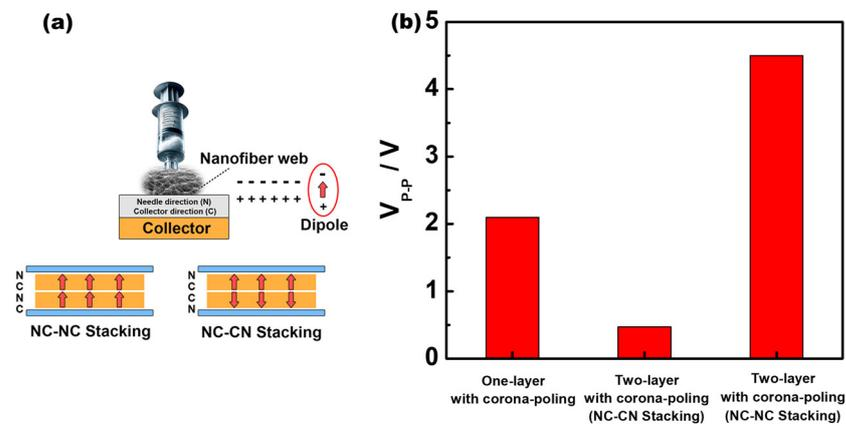
Figure 6. (a) Two kinds of sensors, such as with NC–NC and NC–CN stacking, wherein C and N are the collector and needle directions, respectively. (b) Comparison of  $V_{p-p}$  values of one-layer corona-poled 15 phr BTNP–doped PLA sensor, two-layer corona–poled 15 phr BTNP–doped PLA sensor with NC–CN stacking, and two–layer corona–poled 15 phr BTNP–doped PLA sensor with NC–NC stacking (normal pressure: 5 kgf).
