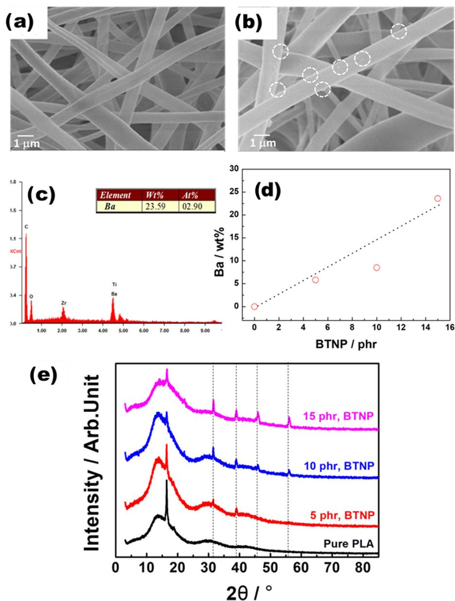
**Figure 2.** (a) FE-SEM micrograph of the pure electrospun PLA nanofiber web. (b) FE-SEM micrograph of the electrospun PLA nanofiber web with 5 phr BTNPs. (c) Typical EDX spectra of the electrospun PLA nanofiber webs with 15 phr BTNPs. (d) Average Ba elements of PLA nanowebs with different BTNP contents. (e) XRD profiles of the prepared samples.
