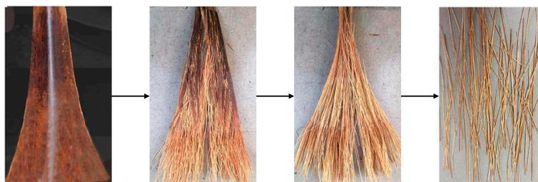
Figure 1. The extraction process of CPFs.
