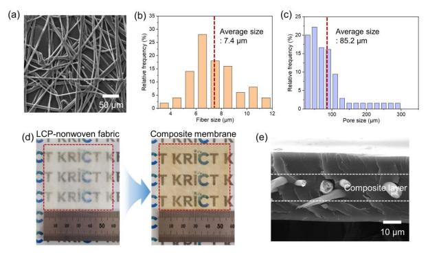
**Figure 3.** (a) Surface SEM image and (b) fiber and (c) pore size distributions of the LCP-nonwoven material. (d) Digital photographs of the surfaces of the LCP-nonwoven material and SPAES50/LCP composite membrane. (e) Cross-sectional SEM image of the SPAES50/LCP composite membrane.
