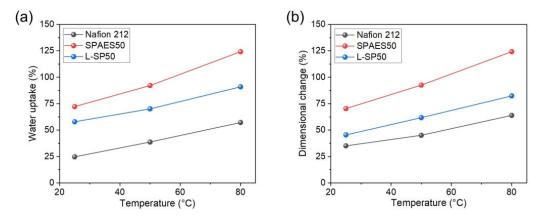
**Figure 4.** (a) Water uptake and (b) volumetric dimensional changes of the Nafion 212, SPAES50, and L-SP50 membranes at 25, 50, and 80  $^{\circ}$ C in water.
