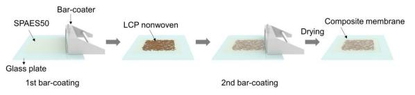
**Figure 2.** Schematic diagram of the preparation of the SPAES50/liquid crystal polymer (LCP) nonwoven composite membranes using a bar-coating method.
