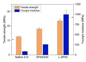
**Figure 5.** Tensile strengths and Young's moduli of the Nafion 212, SPAES50, and L-SP50 membranes at room temperature under wet conditions.
