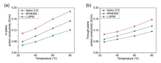
**Figure 6.** Proton conductivities of the Nafion 212, SPAES50, and L-SP50 membranes in (**a**) the in-plane and (**b**) the through-plane directions at 25–80 °C in water.
