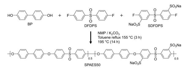
**Figure 1.** Synthetic scheme of the sulfonated poly(arylene ether sulfone) copolymer with a degree of sulfonation of 50 mol% (SPAES50).
