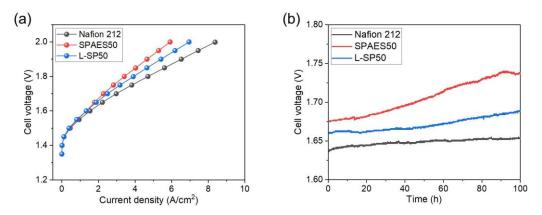
**Figure 7.** (a) PEMWE single-cell performances of the Nafion 212, SPAES50, and L-SP50 membranes (operating temperature: 80 °C; potential range: 1.25-2.0 V; active area:  $5 \text{ cm}^2$ ). (b) Voltage changes in the prepared membranes when a constant current density of  $2 \text{ A/cm}^2$  was applied to the cell for 100 h.
