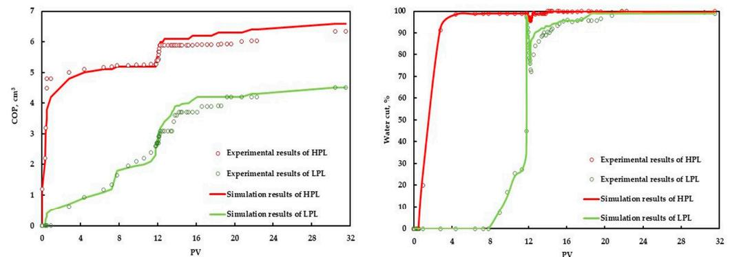
Figure 11. History matching results of the gel flooding experiment.
