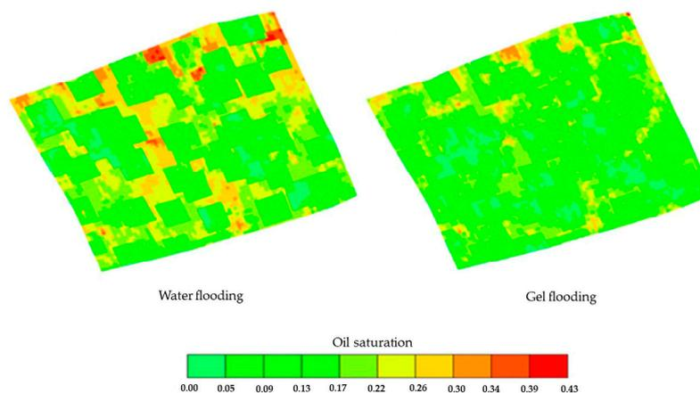
**Figure 18.** The remaining oil saturation distribution comparison between the optimal gel flooding scheme and water flooding.
