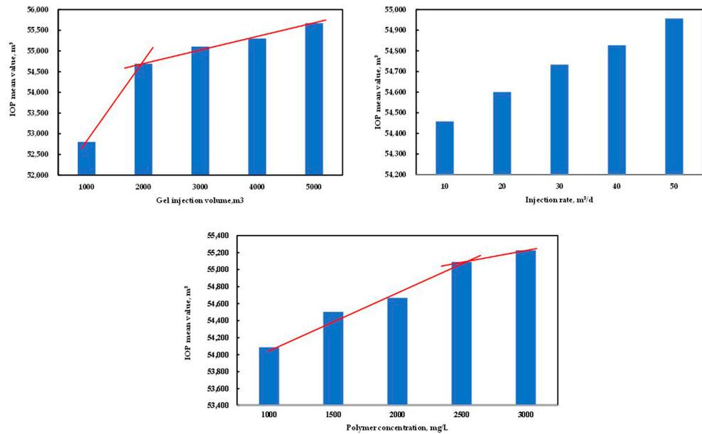
Figure 16. The IOP mean value of the gel injection volume, the injection rate, and the polymer concentration.
