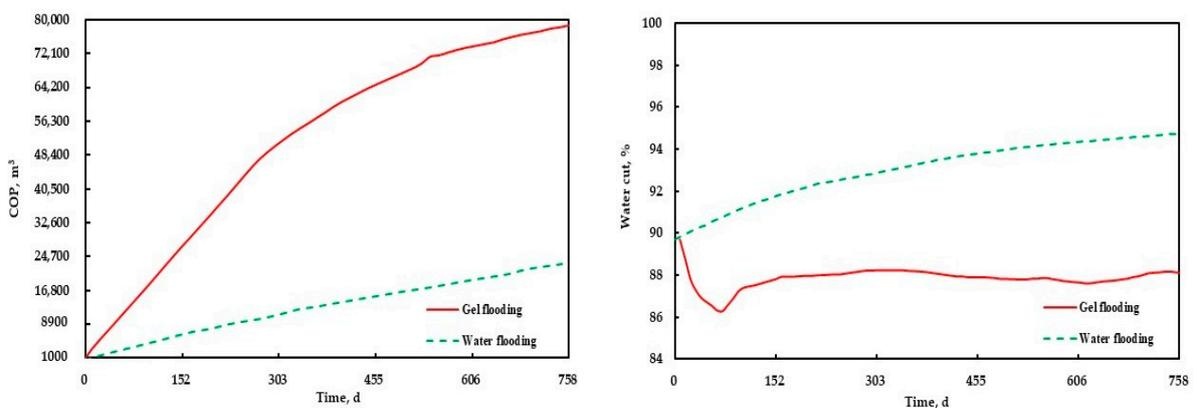
Figure 17. The COP and water cut prediction comparison between the optimal gel flooding scheme and water flooding.
