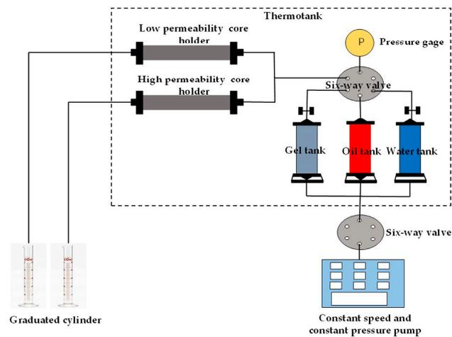
**Figure 3.** Schematic diagram of the gel flooding experimental device.
