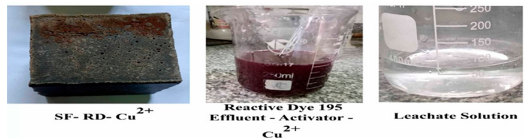
Figure 3. Solidification of a mixture from copper (II) ions and reactive red 195 dyeing bath effluent with slag-FA-based geopolymer mix after 7 days of curing condition.
