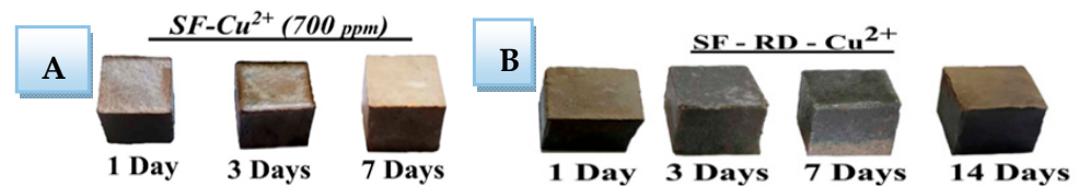
Figure 2. Visual observation of different slag-FA-based geopolymer mixes activated by NaOH and Na 2 SiO 3 after different periods of water curing, (A) SF-Cu 2+ and (B) SF-RD-Cu 2+ .
