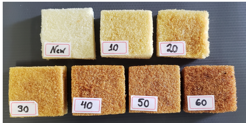
Figure 6. Difference in the PUF color after the ageing process.
