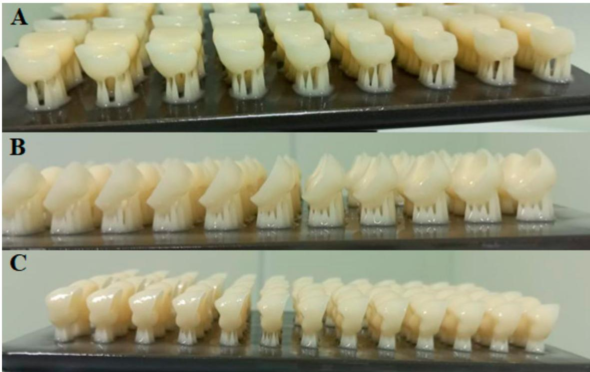
**Figure 5.** The 3D-printed specimens with different orientations for ASIGA. (A) 0-degree, (B) 45-degree, and (C) 90-degree (scale bar 5 mm).
