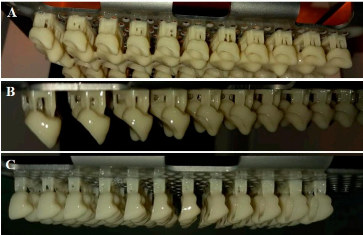
**Figure 4.** (A–C). The 3D-printed specimens with different orientations for NextDent (A) 0-degree, (B) 45-degree, and (C) 90-degree (scale bar 5 mm).
