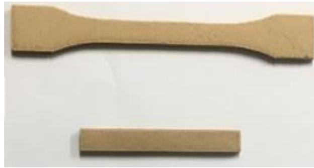
**Figure 2.** The printed ARP/PLA samples.
