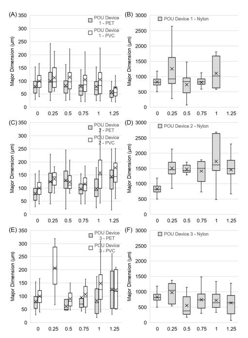
**Figure 4.** Change in size distribution of the major dimensions of PET, PVC, and nylon microplastics as a function of the increasing rated treatment capacity for all three POU devices. X represents the mean and lines represent the maximum, 3rd quartile, median, 1st quartile, and minimum values, from top to bottom.
