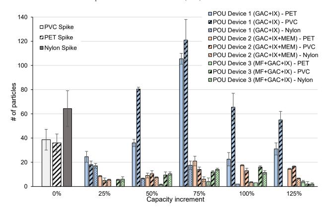
**Figure 3.** Mean microplastic particles or fibers in POU effluent as a function of rated treatment capacity. Vertical bars represent  $\pm$  one standard deviation (n = 2).
