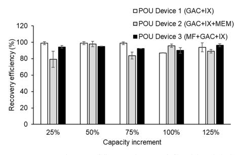
**Figure 2.** Mean particle recovery following each 1 L sample filtered through duplicates of POU Device 1 (GAC + IX), POU Device 2 (GAC + IX + MEM), and POU Device 3 (MF + GAC + IX). Vertical bars represent  $\pm$  one standard deviation (n = 2).
