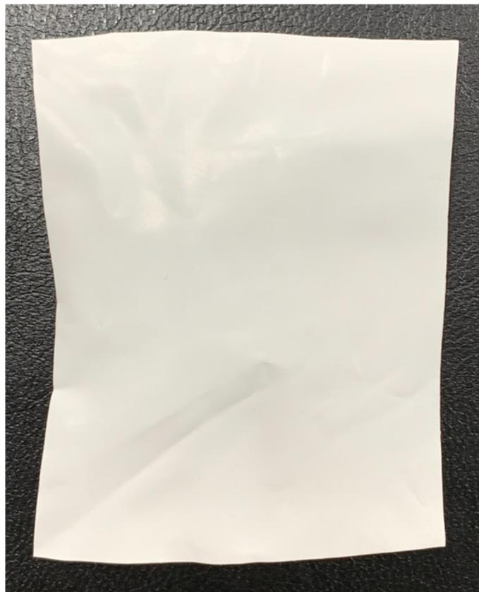
**Figure A1.** The photo of a PVDF membrane prepared by immersing the PVDF/NMP (20 wt% of PVDF) solution in water.
