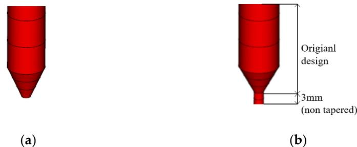
Figure 19. Pin-point gate shape. (a) Original design; (b) non-tapered modified design.
