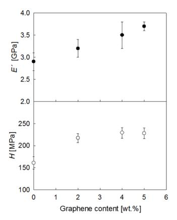
**Figure 10.** Storage modulus and hardness as a function of graphene content for PET and PET/ graphene fibers.
