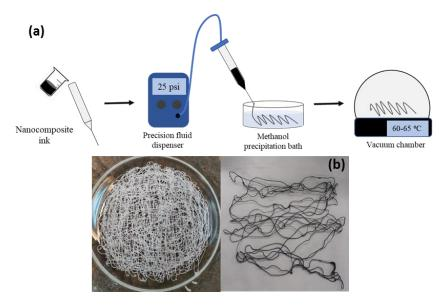
**Figure 3.** (a) Scheme of dry–jet wet–spinning method using a precision fluid dispenser and manually creating the fibers. (b) Photograph of PET (left) and PET/graphene fibers with a loading of 4 wt.% prepared by dry–jet wet spinning.
