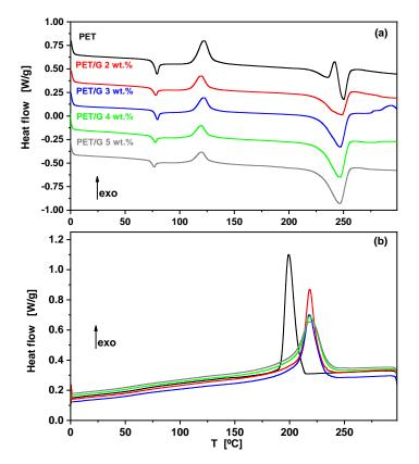
Figure 8. DSC heating scan for PET fibers (a) and subsequent cooling scan (b).
