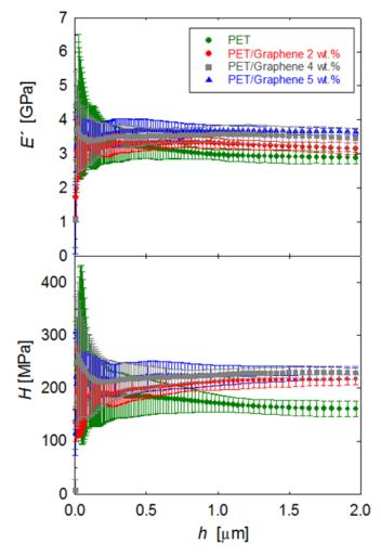
**Figure 9.** *E* ´ and *H* behavior as a function of indent displacement, for PET and PET/graphene fibers.
