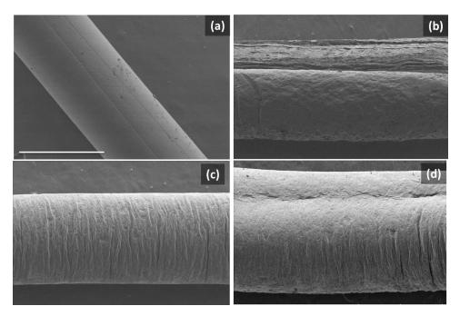
**Figure 4.** SEM images of the surfaces of dry-jet-wet-spinning-produced fibers: (**a**) PET and PET/ graphene with loadings of (**b**) 2 wt.%, (**c**) 4 wt.% and (**d**) 5 wt.%. Scale bar in (**a**) applies to all images and corresponds to 500 microns.
