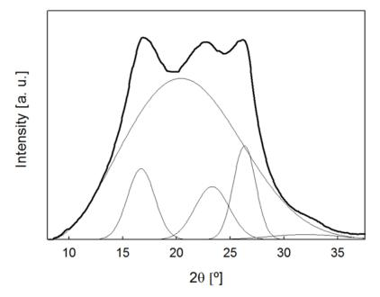
**Figure 2.** Intensity profile as a function of diffraction angle for a PET/graphene 5 wt.% fiber with 575 µm radius. The curve is separated into an amorphous halo and several crystalline peaks.
