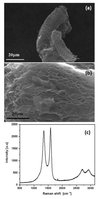
**Figure 1.** SEM images at different magnifications (**a**,**b**) and Raman spectrum (**c**) of the G employed for PET/G nanocomposite fibers.
