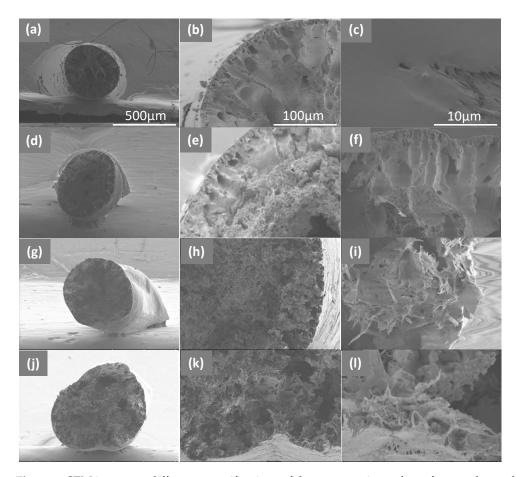
**Figure 5.** SEM images at different magnifications of the cross-sections of cryofractured samples of PET (**a**–**c**) and PET/graphene with loadings of 2 wt.% (**d**–**f**), 4 wt.% (**g**–**i**) and 5 wt.% (**j**–**l**). Scale bar in (**a**–**c**) applies to the images in the same column.
