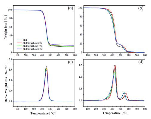
**Figure 6.** TGA and dTGA curves for PET and PET/graphene nanocomposites with different graphene loadings under nitrogen (**a**,**c**) and air (**b**,**d**) atmospheres. Heating scan =  $5 \degree \text{C} \cdot \text{min}^{-1}$ .
