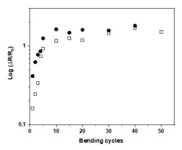
**Figure 11.** Variation in the resistance of PET/G fibers with different graphene loadings with the number of bending cycles (open squares and full circles correspond to loadings of 4 wt.% and 5 wt.%, respectively).
