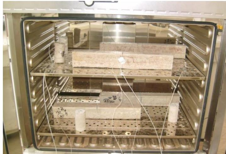
**Figure 4.** Temperatures control through installation of thermocouples.
