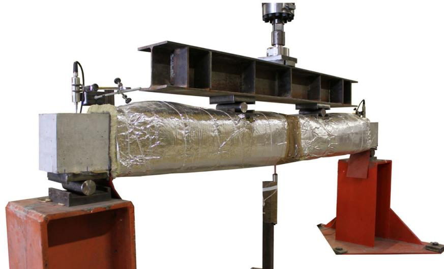
**Figure 4.** General view of experimental setup.
