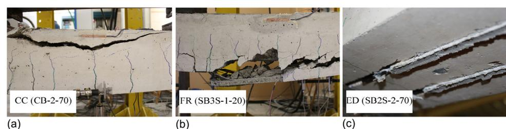
**Figure 10.** Representative failure modes of the specimens. (a) CC (concrete crushing); (b) FR (FRP rupture); and (c) ED (end debonding).
