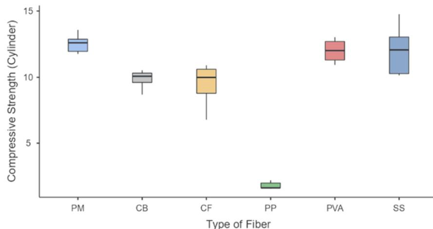
**Figure 3.** Compressive strength of fiber-reinforced geopolymer.
