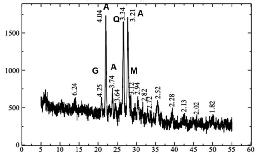
Figure 1. Product characterization of PM samples by XRD.
