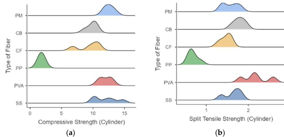
**Figure 6.** Density plot of responses for (a) compressive strength and (b) split-tensile strength.
