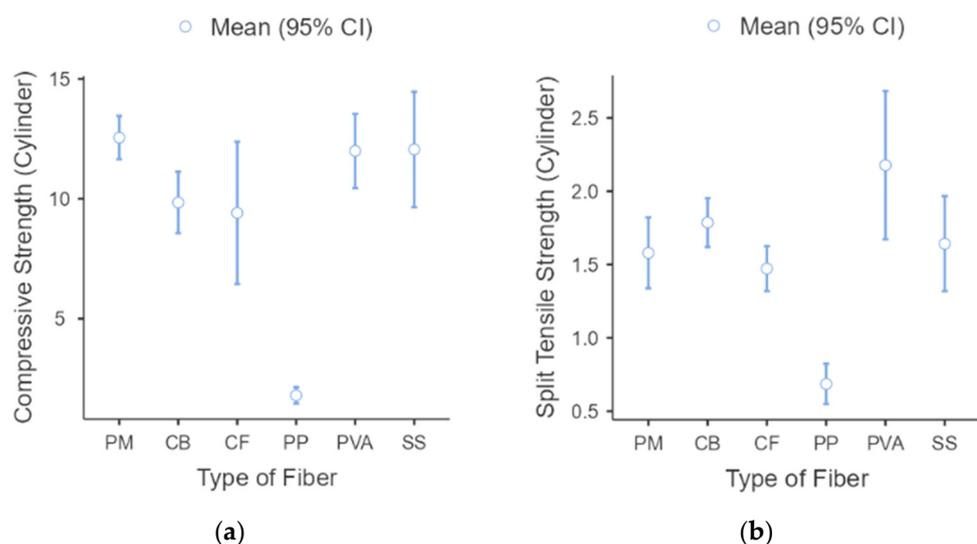
**Figure 7.** Box plot for FRG samples (a) compressive strength and (b) split-tensile strength.
