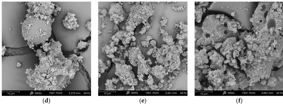
**Figure 10.** SEM Images of fiber-reinforced GP samples: (a) CB fibers, (b) CF fibers, (c) SS fibers (d) PP fibers, (e) PVA fibers, and (f) Plain Mortar (PM).
