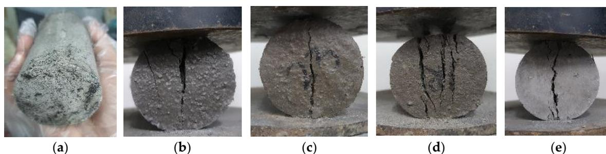
**Figure 4.** Geopolymer mortar with cracked split-tensile cylindrical samples of (a) PP fibers, (b) SS fibers, (c) PVA fibers, (d) CB fibers, and (e) Carbon fibers (CF).
