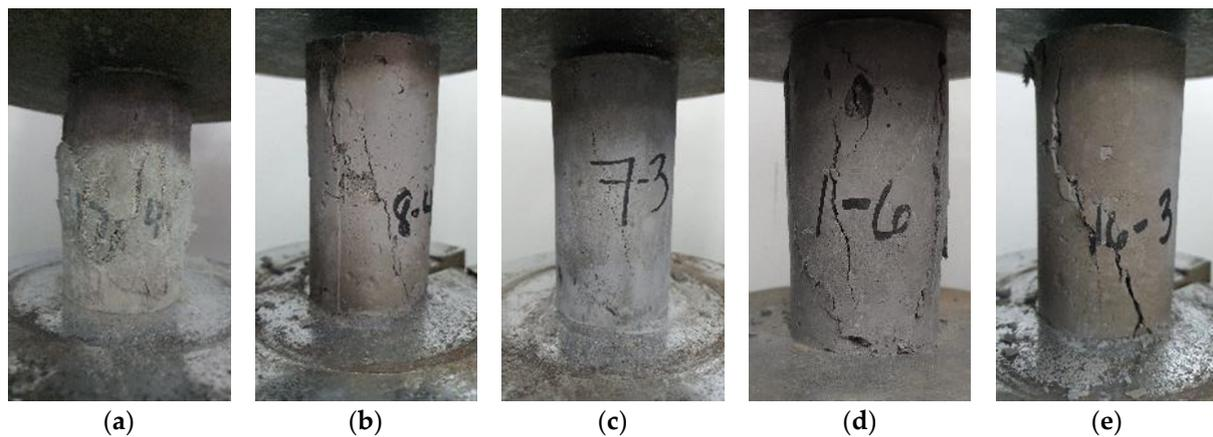
**Figure 2.** Geopolymer mortar with cracked cylindrical samples of (a) PP fibers, (b) SS fibers, (c) PVA fibers, (d) CB fibers, and (e) Carbon fibers (CF).
