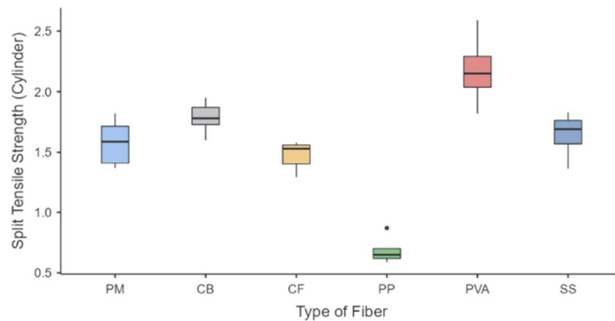
**Figure 5.** Split Tensile Strength of fiber-reinforced geopolymers.
