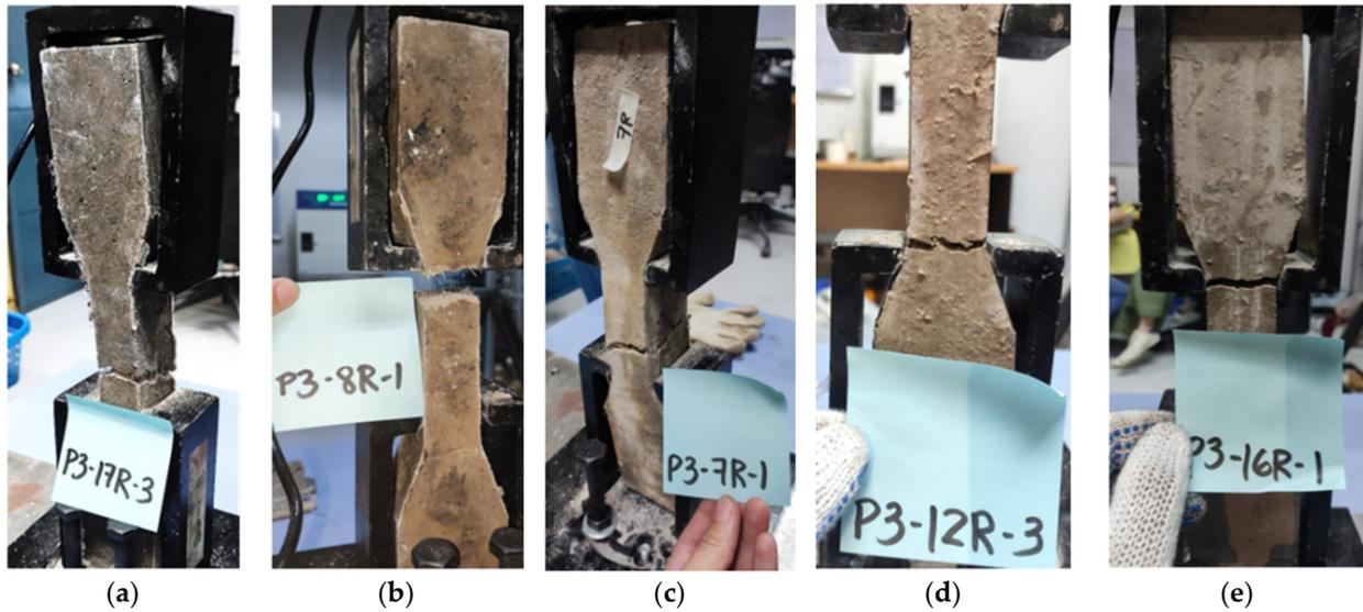
**Figure 8.** Geopolymer mortar with cracked dog-bone samples of (a) PP fibers, (b) SS fibers, (c) PVA fibers, (d) CB fibers, and (e) Carbon fibers (CF).
