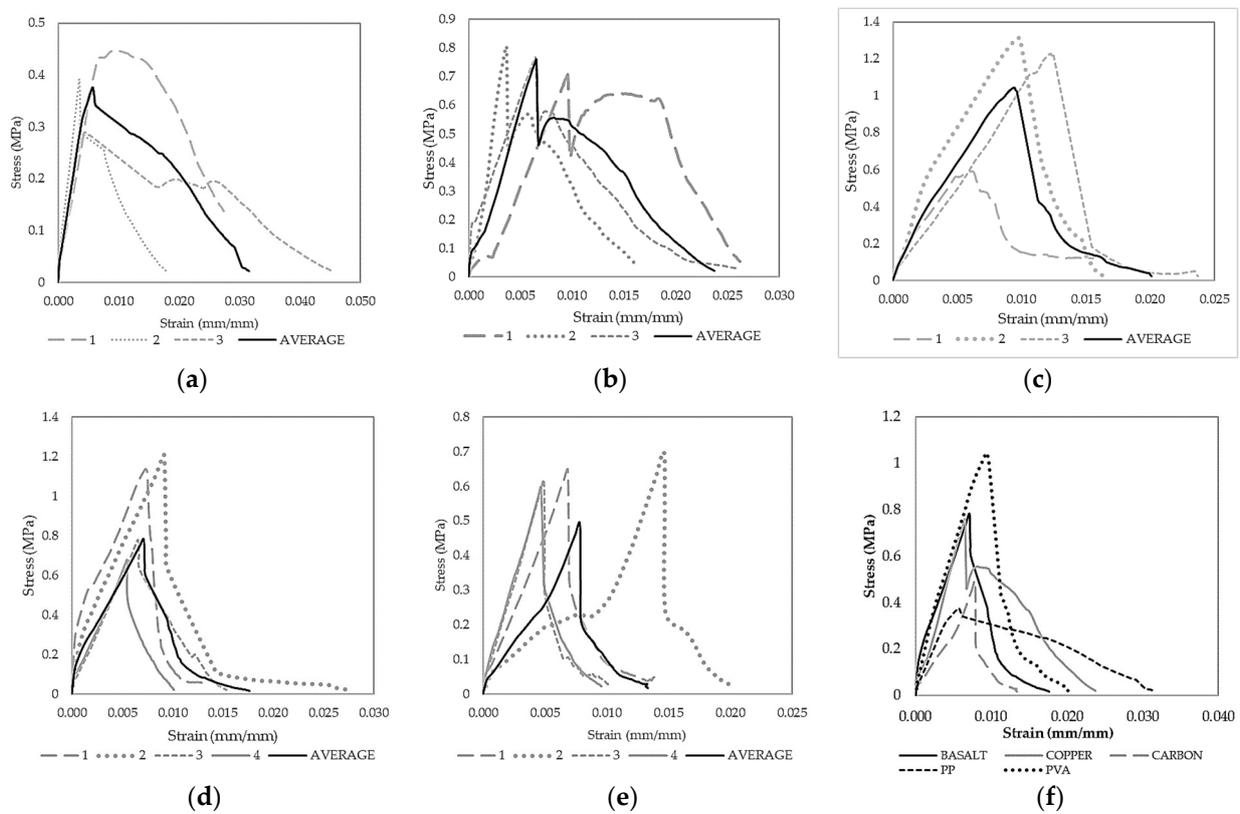
**Figure 9.** Geopolymer mortar with the stress–strain diagram of (a) PP fibers, (b) SS fibers, (c) PVA fibers, (d) CB fibers, (e) Carbon fibers (CF), and (f) summary of all fiber types.
