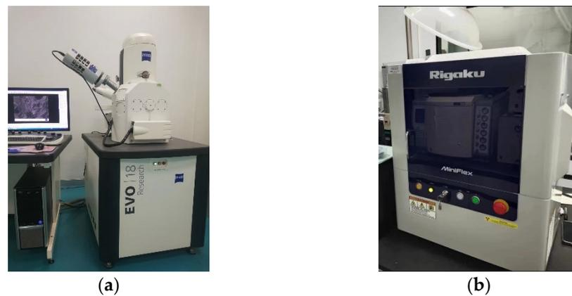
**Figure 7.** (a) Low vacuum scanning electron microscope equipment and (b) X-ray diffraction instrument.
