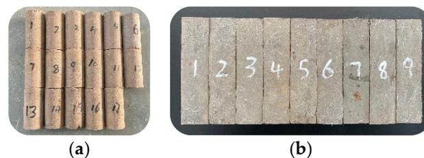
**Figure 5.** Composite material samples. (a) Uniaxial compression test samples (b) Three-point bending test sample.
