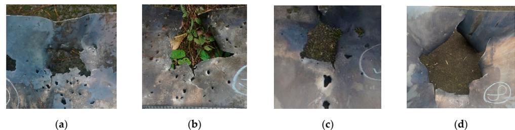
**Figure 13.** Damage on the front side of the aluminum target plate: (a) No. 3, (b) No. 4, (c) No. 5, and (d) No. 8.
