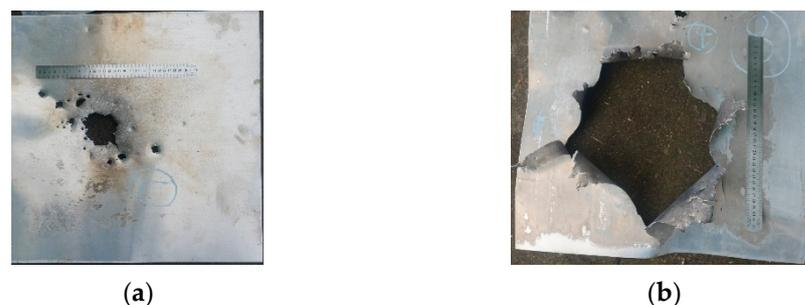
**Figure 12.** Damage of two kinds of projectiles to the aluminum target plate: (a) No. 7, conventional projectile; (b) No. 8 PELE projectile filled with reactive material.
