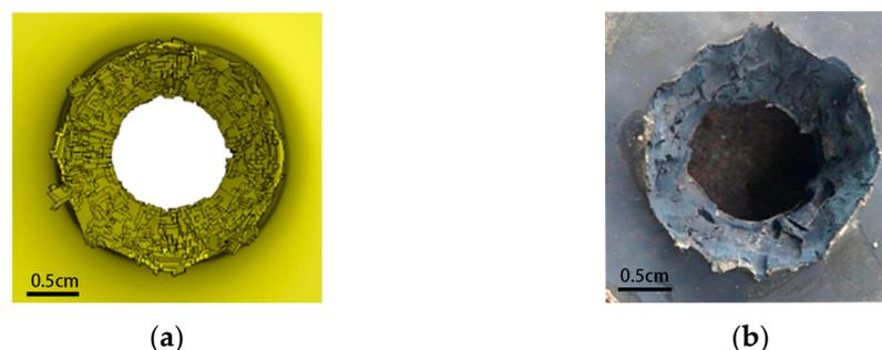
**Figure 10.** Bullet hole shape: (a) numerical simulation and (b) test result.
