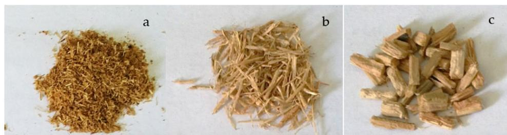
**Figure 2.** The OPF particles with different sizes (a) fine, (b) medium, (c) coarse.
