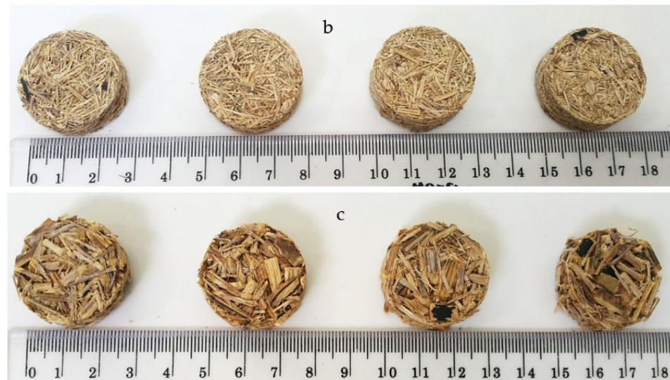
**Figure 3.** Acoustic test samples with different particle sizes and densities (a) fine, (b) medium, (c) coarse.
