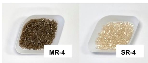
**Figure 3.** Generated recycled pellets obtained after the 4th reprocessing cycle.
