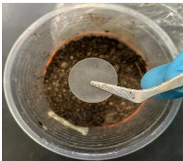
Figure 17. Appearance of pure 3D printed plant-based film before the soil burial test.
