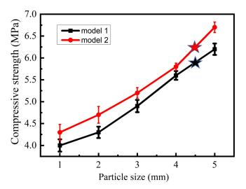
**Figure 6.** The effect of soil particle size on compressive strength of consolidated soil columns. The black star represents the compressive strength of sample 6; The red star represents the compressive strength of sample 12.
