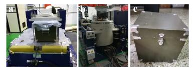
**Figure 2.** Vibration resistance testing of consolidated soil columns. (a) LS437A/BT900M(4T) Vibration Table; (b) MPA3324/H1248A (10T) vibration table; (c) Sample box.
