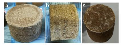
**Figure 3.** Prepared consolidated soil column. (a) Front of consolidated soil column model 2; (b) Sides of consolidated soil column model 2; (c) Front of consolidated soil column model 1.
