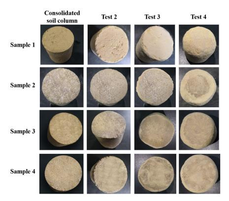
Figure 11. Wear state of consolidated soil columns tested using Method 2.
