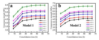
**Figure 7.** The effect of consolidation time of adhesive on the compressive strength of consolidated soil columns. (a) Effect of different consolidation times on consolidation strength in Model 1 of consolidated soil column; (b) Effect of different consolidation times on consolidation strength in Model 2 of consolidated soil column.
