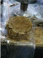
**Figure 5.** Test method for compressive strength of consolidated soil columns. (a) Compressive strength testing of consolidated soil columns; (b) Consolidated soil column after compression.
