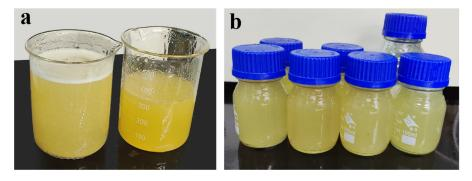
**Figure 1.** KGM/CA/PVA ternary blend adhesive. (a) Main adhesive of prepared KGM/CA/PVA polymer adhesive; (b) KGM/CA/PVA soil consolidation agent with additives added.
