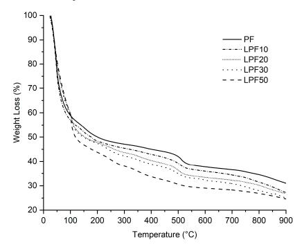
Figure 5. Thermogram results for the different resins.
