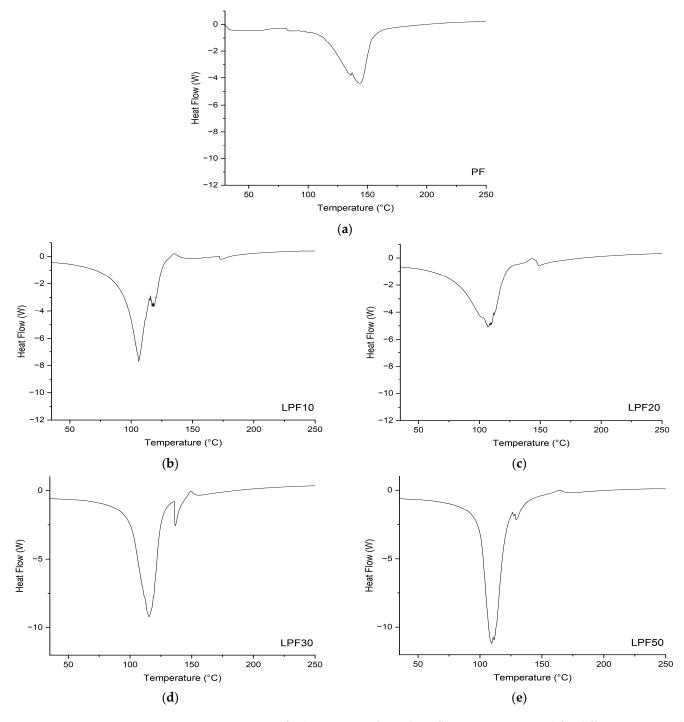
**Figure 4.** Diagrams of calorimetry analyses (heat flow per temperature) for different resins under study: (a) PF, (b) LPF10, (c) LPF20, (d) LPF30 and (e) LPF50.
