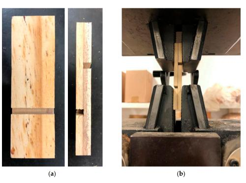
Figure 1. Shear strength test in the glue line: (a) specimens, and (b) test in operation.
