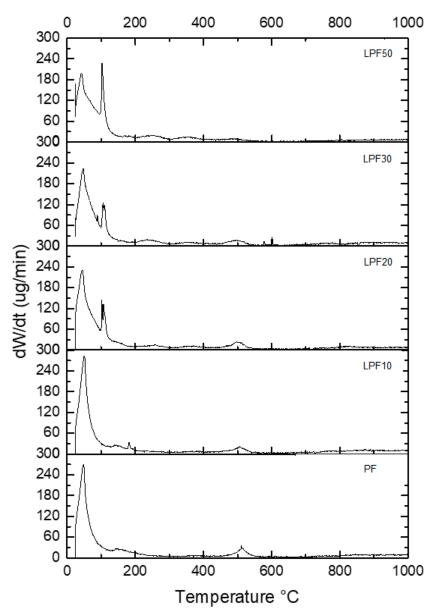
from 400 °C to 600 °C; and above 600 °C. Most of the thermal events occur in the first stage and explain the lower stability of the LPF resin compared to PF.
