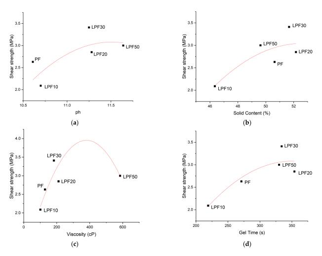
Figure 3. Development of tensile shear strength of different resins as a function of: (a) pH, (b) solid content, (c) viscosity, and (d) gel time.
