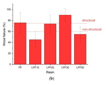
Figure 2. Influence of different resins on: (a) tensile shear strength, and (b) wood failure.
