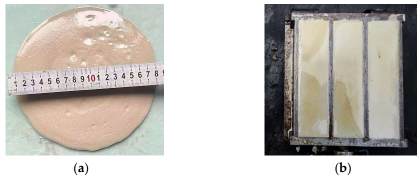
Figure 6. Pre-test of water binder ratio. (a) Fluidity; (b) Water secretion.
