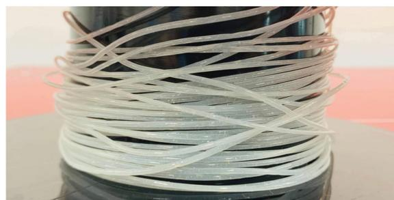
**Figure 4.** PLA nanocomposite filament spool.
