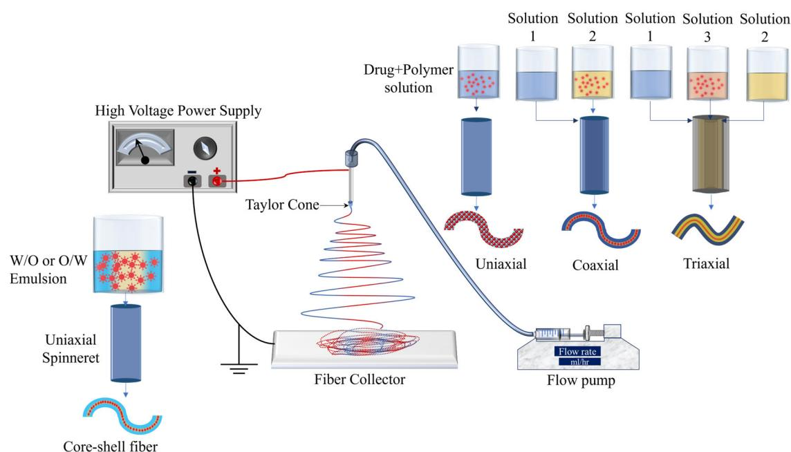
**Figure 3.** Schematic of electrospinning and its types.
