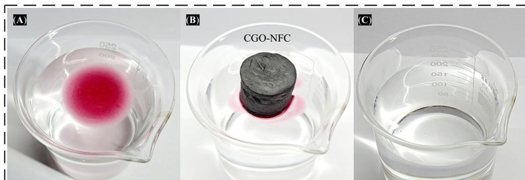
**Figure 14.** Absorption test of CGO-NFC in carmine red-dyed engine oil: (A) before addition of CGO-NFC, (B) during absorption with CGO-NFC, and (C) after absorption.
