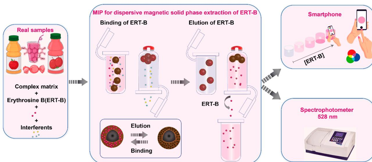
**Figure 5.** Schematic illustration of the application of magnetic MIPda as an adsorbent in SPE for optical detection of ERT. Permission granted from the corresponding author of reference [27] (MDPI).
