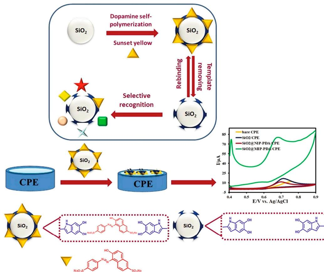
**Figure 4.** Fabrication process of sunset-yellow-imprinted  $\text{SiO}_2$ @PDA NPs electrochemical sensor and its application to detect sunset yellow. Reused, with permission from Elsevier publishers, from reference [48].
