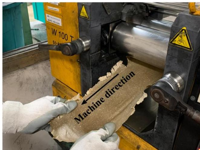
**Figure 2.** Fiber alignment on a two-roll mill during the uniaxial composite prepreg preparation.
