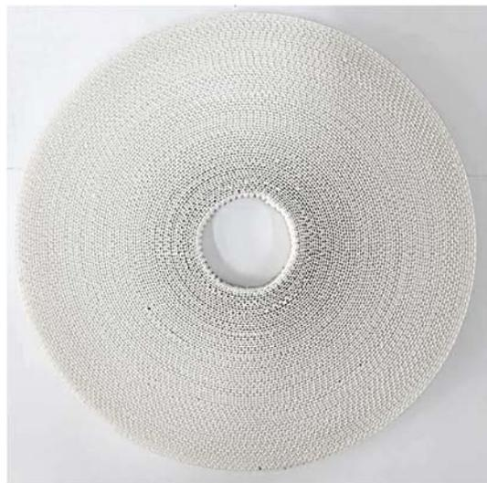
**Figure 1.** Photograph of the substrate of desiccant wheels.
