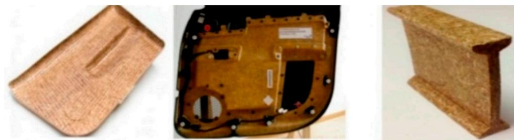
**Figure 11.** Automotive parts developed from natural-fibre-based composites. Reproduced from [113].
