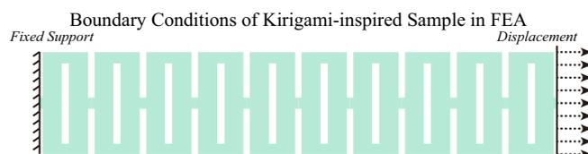
**Figure 4.** Illustration of FEA settings. The boundary conditions (fixed support and displacement) are indicated.
