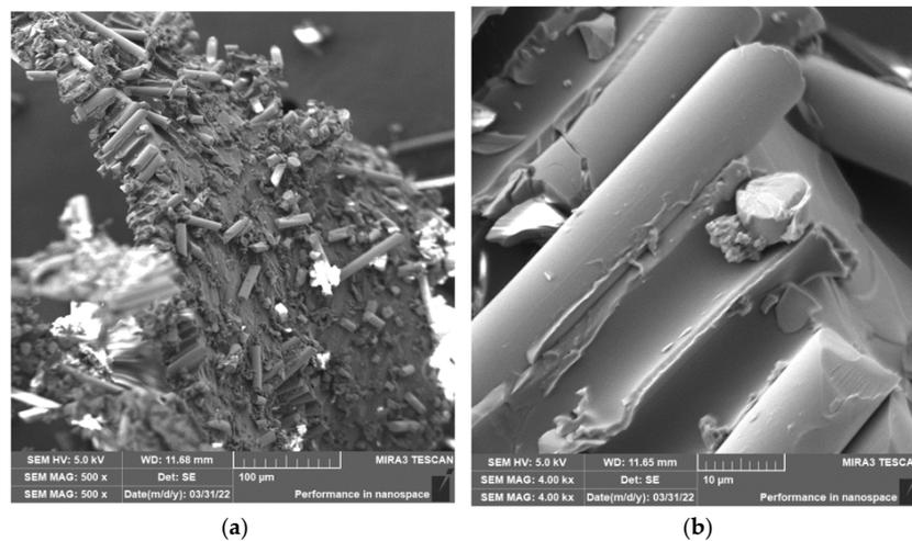
**Figure 16.** Glass fibers in epoxy resin. (a) Detailed chip image after drilling with broken glass fibers and matrix particles ( $n = 1500$  rpm,  $D = 5.0$  mm, and  $f_n = 0.2$  mm/min). (b) Close-up of glass fibers with typical fractures.
