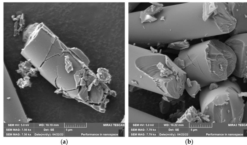
**Figure 17.** Glass fibers after removing the epoxy matrix. (a) Image of glass fiber destruction after drilling ( $n = 1000$  rpm,  $D = 9.8$  mm, and  $f_n = 0.2$  mm/min). (b) A close-up of the characteristic fracture surfaces of glass fibers after drilling ( $n = 1500$  rpm,  $D = 5.0$  mm, and  $f_n = 0.2$  mm/min).
