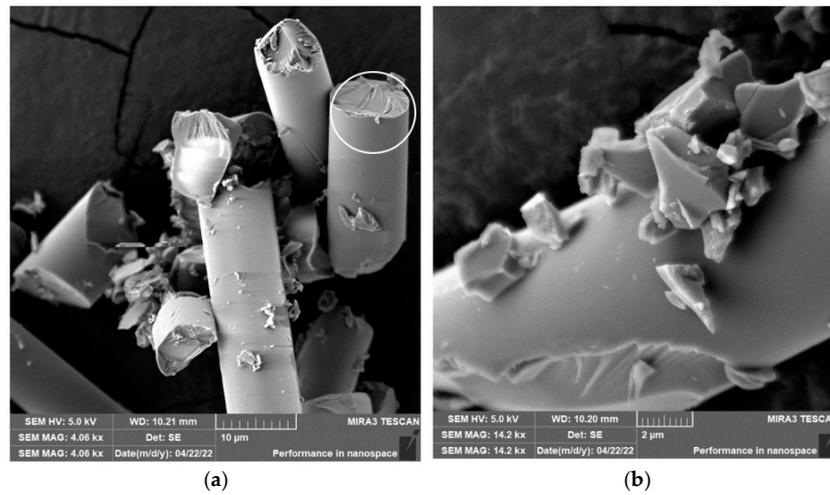
**Figure 14.** Glass fibers after removing the epoxy matrix. (a) Image of glass fibers and fragments created after milling ( $n = 1000$  rpm,  $a_p = 2$  mm, and  $v_f = 100$  mm/min) with a characteristic brittle fracture in a white circle. (b) Close-up of glass fibers and their fragments.
