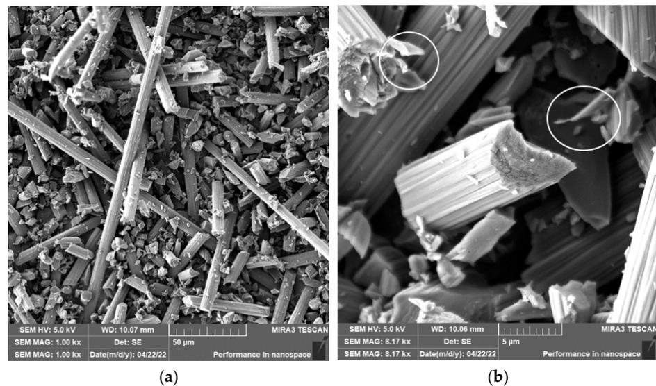
**Figure 11.** Carbon fibers after removing the epoxy matrix. (a) Image of carbon fibers and their fragments formed after grinding ( $n = 2400$  rpm,  $a_p = 0.2$  mm, and  $v_f = 200$  mm/min). (b) A detailed image of carbon fibers and their fragments in a white circle, including the nature of fracture surfaces.
