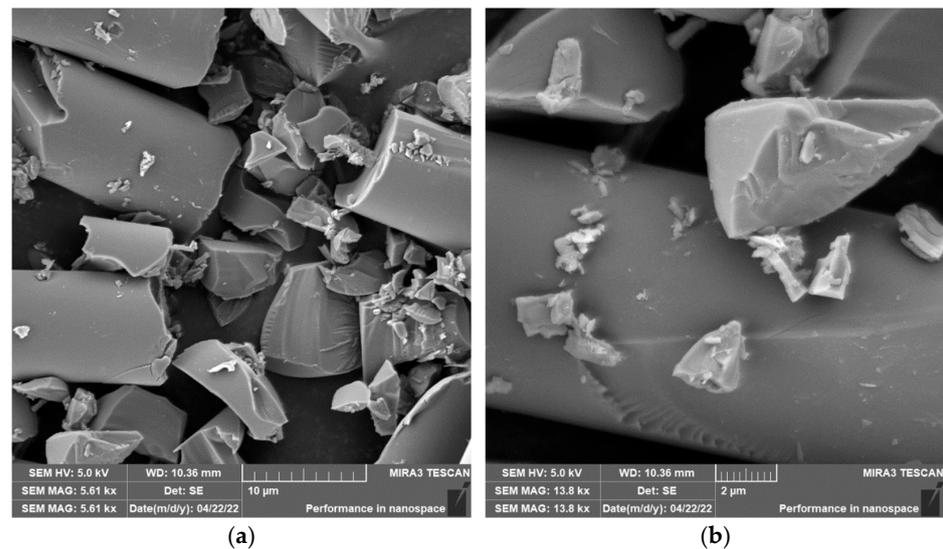
**Figure 20.** Glass fibers after removing the epoxy matrix. (a) Image of destroyed glass fibers after grinding ( $n = 2400$  rpm,  $a_p = 0.2$  mm, and  $v_f = 200$  mm/min). (b) Close-up of sub-micrometer glass fiber particles.
