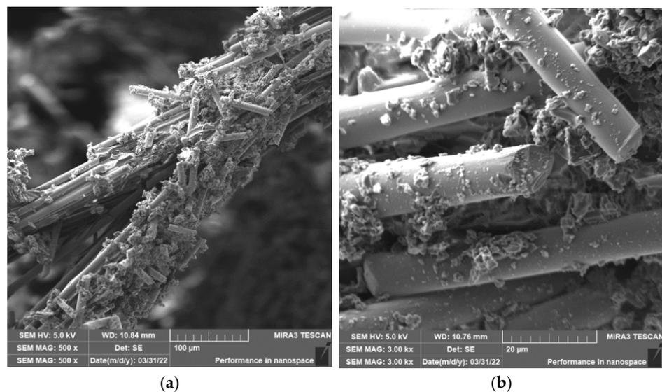
**Figure 13.** Glass fibers in epoxy resin. (a) Image of the chip after milling ( $n = 1000$  rpm,  $a_p = 1$  mm, and  $v_f = 100$  mm/min) with broken glass fibers and matrix particles. (b) Close-up of broken glass fibers with matrix particles.
