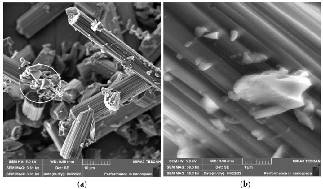
**Figure 7.** Carbon fibers after removing the epoxy matrix. (a) Image of carbon fibers and their fragments formed after drilling in a white circle ( $n = 1500$  rpm,  $D = 5.0$  mm, and  $f_n = 0.2$  mm/min). (b) A close-up of the surface of a carbon fiber with sub-micrometer particles formed during its destruction.
