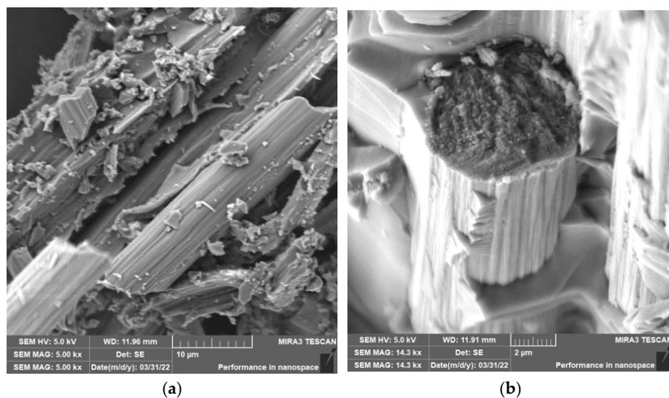
**Figure 10.** Carbon fibers in an epoxy matrix. (a) Image of carbon fibers and their fragments after grinding ( $n = 2400$  rpm,  $a_p = 0.2$  mm, and  $v_f = 200$  mm/min). (b) Close-up of the fracture surface of carbon fiber surrounded by an epoxy matrix.
