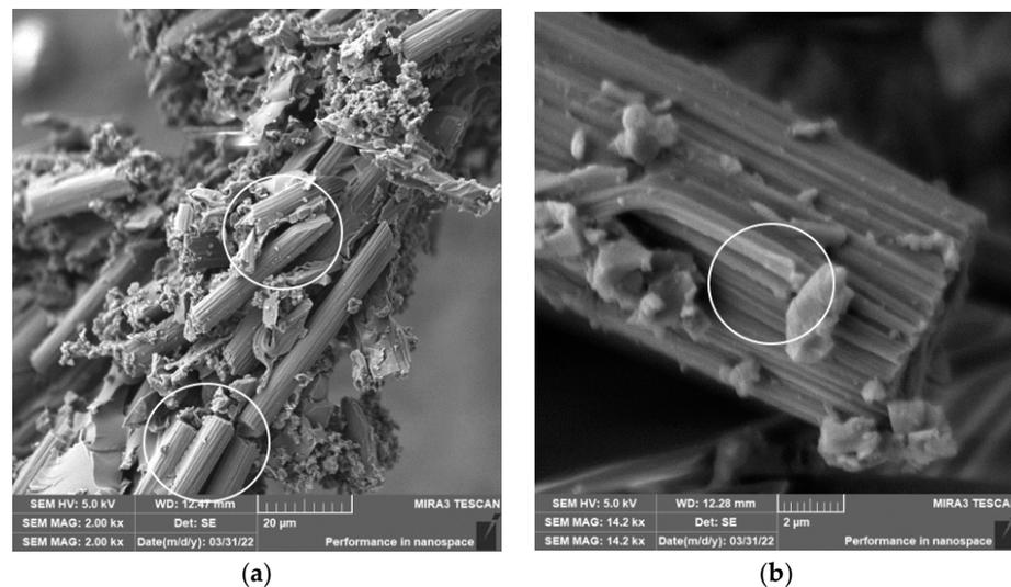
**Figure 4.** Carbon fibers in an epoxy matrix. (a) Detailed image of a chip after milling ( $n = 1000$  rpm,  $a_p = 1$  mm, and  $v_f = 100$  mm/min) with broken carbon fibers and matrix particles—in white circles are directions of fractures—perpendicular and at an angle to the fiber axis. (b) Close-up of the surface longitudinal failure of carbon fiber with matrix particles in the white circle.
