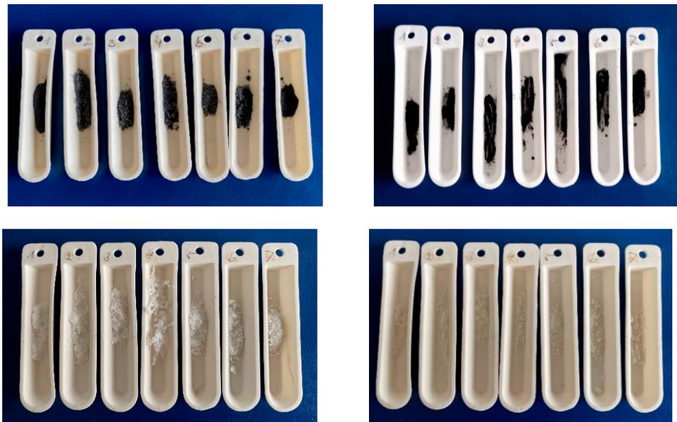
**Figure 2.** Illustrative image of chips generated during the selected machining process (left) and after removing the epoxy matrix by firing it (right) for carbon fiber (top) and glass fiber (bottom) systems.
