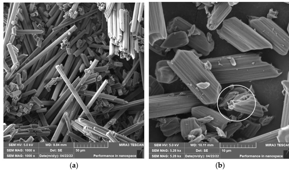
**Figure 5.** Carbon fibers after removing the epoxy matrix. (a) Image of carbon fibers formed after milling ( $n = 1000$  rpm,  $a_p = 2$  mm, and  $v_f = 100$  mm/min) with an example of length variability. (b) A close-up of the nature of the direction of fractures and the sizes of the carbon fiber fragments after milling ( $n = 1000$  rpm,  $a_p = 1$  mm, and  $v_f = 100$  mm/min) in a white circle.
