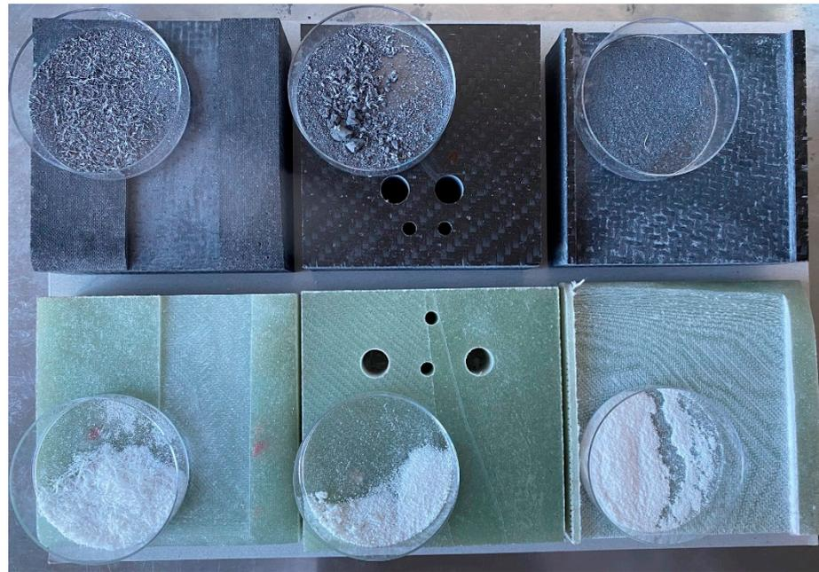
**Figure 1.** Image of prepared composite samples and chips from them during the machining processes of milling, drilling, and grinding (from left to right). Carbon fiber composite samples (upper row), glass fiber composite samples (lower row).
