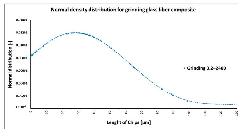
**Figure 18.** Dependency of frequency of occurrence and lengths of destroyed fibers concerning grinding technology.
