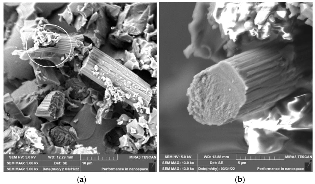
**Figure 8.** Carbon fibers in an epoxy matrix. (a) Image of carbon fiber fragments after drilling ( $n = 1000$  rpm,  $D = 9.8$  mm, and  $f_n = 0.2$  mm/min) with compact matrix and matrix particles visible in a white circle. (b) A detailed image of the fracture surface character of the carbon fiber after drilling ( $n = 1500$  rpm,  $D = 9.8$  mm, and  $f_n = 0.2$  mm/min).
