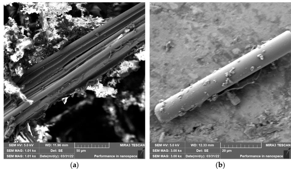
**Figure 19.** Glass fibers in epoxy resin. (a) Image of a bundle of glass fibers and matrix particles after grinding ( $n = 2400$  rpm,  $a_p = 0.2$  mm, and  $v_f = 200$  mm/min). (b) Close-up of the glass fiber and matrix particles.
