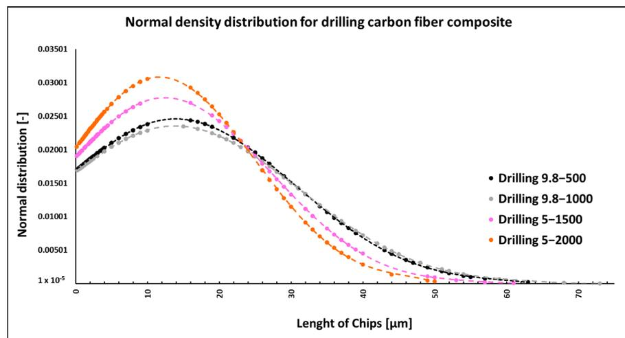
**Figure 6.** Dependencies of frequency of occurrence and lengths of destroyed fibers concerning drilling technology.
