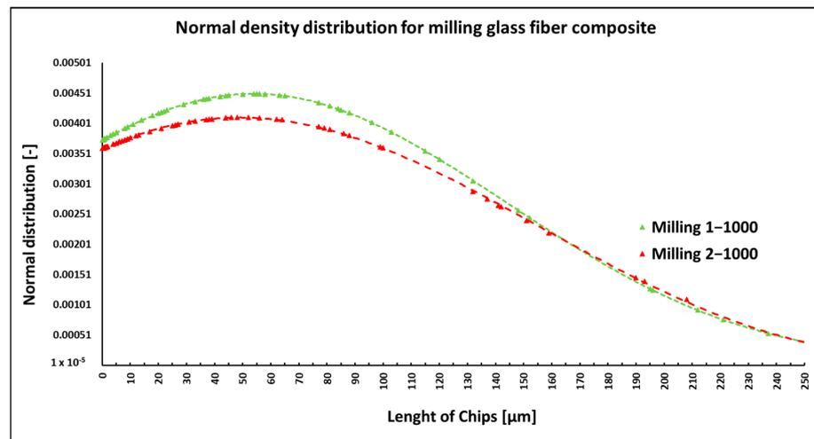
**Figure 12.** Dependencies of frequency of occurrence and lengths of destroyed fibers concerning milling technology.
