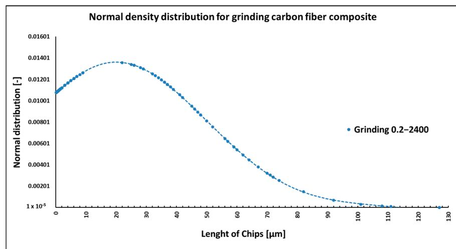
**Figure 9.** Dependencies of frequency of occurrence and lengths of destroyed fibers concerning grinding technology.
