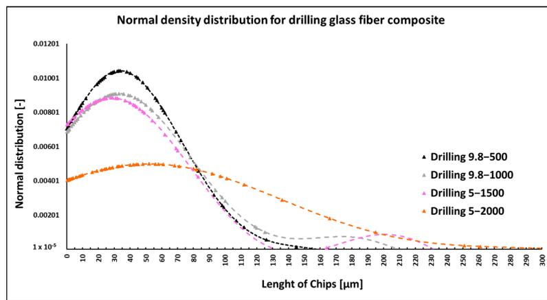
**Figure 15.** Dependencies of frequency of occurrence and lengths of destroyed fibers concerning drilling technology.
