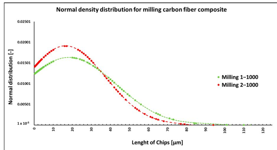
**Figure 3.** Dependencies of frequency of occurrence and lengths of destroyed fibers concerning milling technology.
