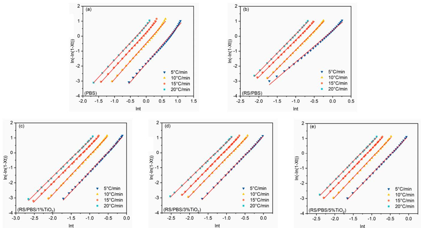
**Figure 4.** Avrami plots of  $\ln[-\ln(1 - X_t)]$  versus  $\ln t$  for the non-isothermal crystallization of (a) PBS, (b) RS/PBS, (c) RS/PBS/1%TiO<sub>2</sub>, (d) RS/PBS/3%TiO<sub>2</sub>, and (e) RS/PBS/5%TiO<sub>2</sub>.
