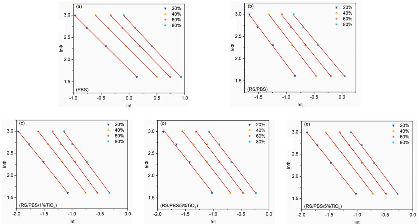
Figure 6. Plots of  $\ln \Phi$  versus  $\ln t$  for (a) PBS, (b) RS/PBS, (c) RS/PBS/1%TiO<sub>2</sub>, (d) RS/PBS/3%TiO<sub>2</sub>, and (e) RS/PBS/5%TiO<sub>2</sub> at different degree of crystallinity.
