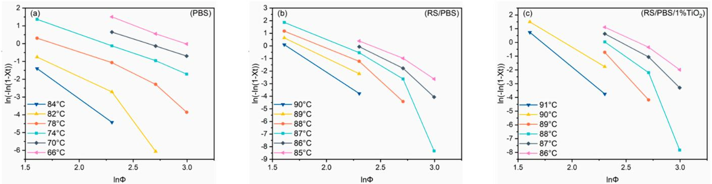
Figure 5. Ozawa plots of  $\ln[-\ln(1-X_T)]$  versus  $\ln \Phi$  for the non-isothermal crystallization of (a) PBS, (b) RS/PBS, and (c) RS/PBS/1%TiO<sub>2</sub>.
