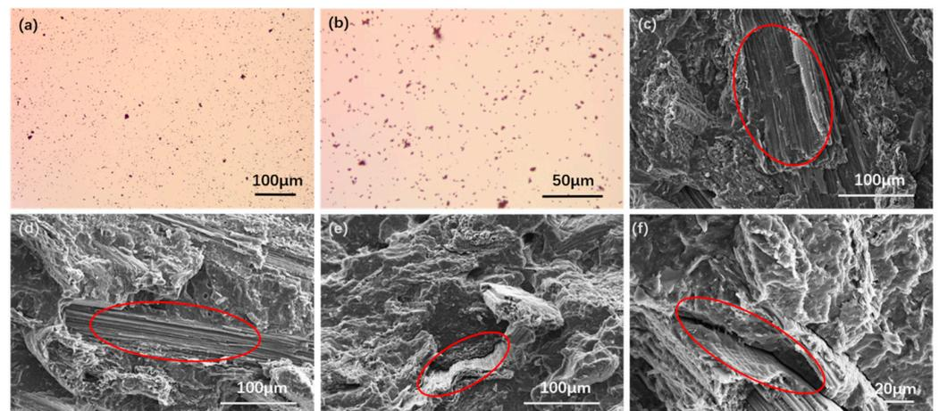
**Figure 9.** Micrograph of  $\text{TiO}_2$  and RS/PBS composites. (a,b)  $\text{TiO}_2$ , (c) RS/PBS, (d) RS/PBS/1% $\text{TiO}_2$ , (e) RS/PBS/3% $\text{TiO}_2$ , and (f) RS/PBS/5% $\text{TiO}_2$ .
