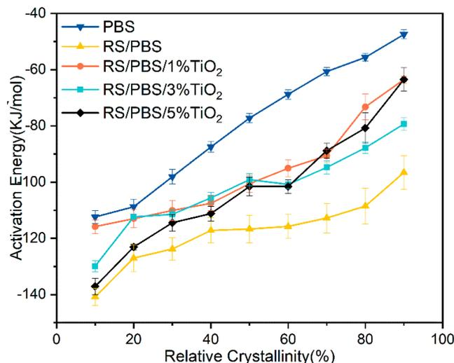
**Figure 7.** Effective activation energy versus the relative degree of crystallinity obtained from Friedman's method for PBS and the composites.
