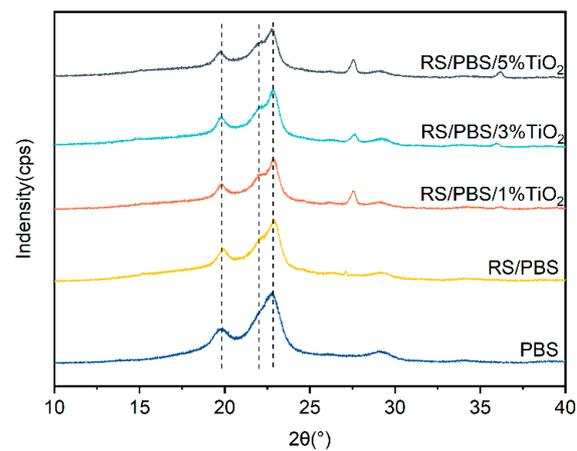
**Figure 8.** XRD patterns of PBS and the composites.
