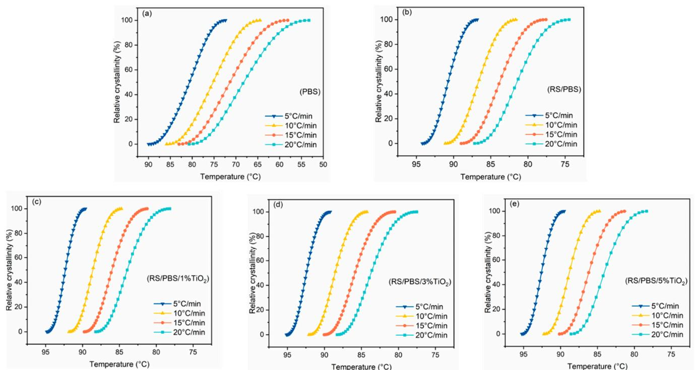
**Figure 2.** The relative crystallinity versus crystallization temperature for (a) PBS, (b) RS/PBS, (c) RS/PBS/1%TiO<sub>2</sub>, (d) RS/PBS/3%TiO<sub>2</sub>, and (e) RS/PBS/5%TiO<sub>2</sub> at various cooling rates.
