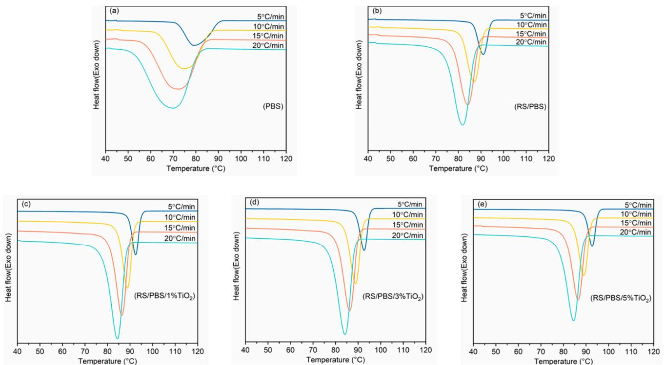
**Figure 1.** Non-isothermal melt crystallization curves of (a) PBS, (b) RS/PBS, (c) RS/PBS/1%TiO<sub>2</sub>, (d) RS/PBS/3%TiO<sub>2</sub>, and (e) RS/PBS/5%TiO<sub>2</sub> under different cooling rates.
