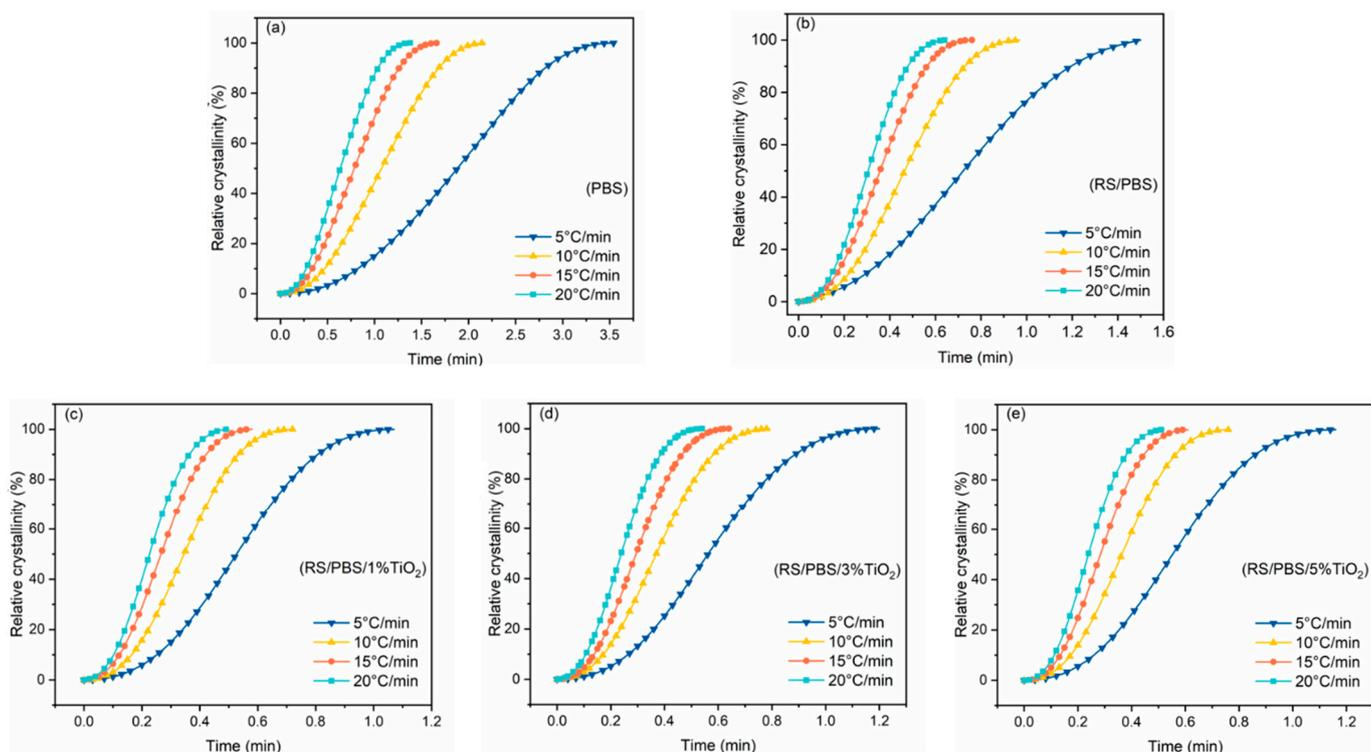
**Figure 3.** The relative crystallinity versus crystallization time for (a) PBS, (b) RS/PBS, (c) RS/PBS/1%TiO<sub>2</sub>, (d) RS/PBS/3%TiO<sub>2</sub>, and (e) RS/PBS/5%TiO<sub>2</sub> at various cooling rates.
