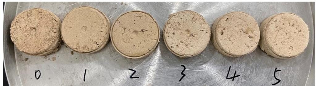
**Figure 1.** The appearance of the loess columns containing 0%, 1%, 2%, 3%, 4%, and 5% PCF (based on loess weight), respectively.
