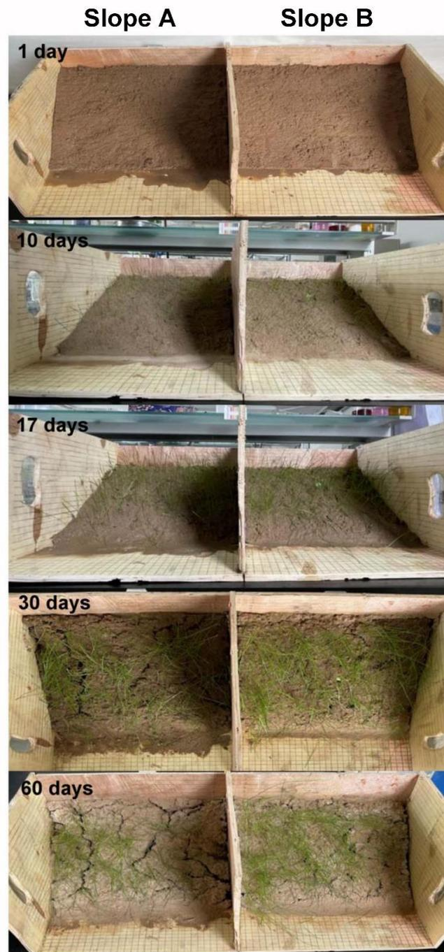
**Figure 13.** Digital photographs of vegetation (*Cyperaceae*) in loess slopes treated without PCF (Slope A) and with 2 wt% PCF (Slope B).
