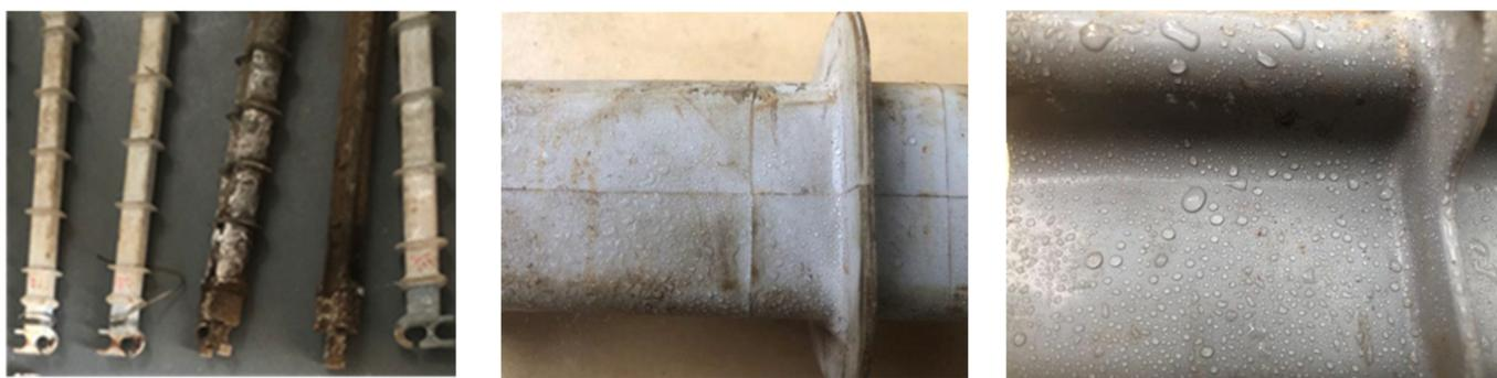
**Figure 3.** Morphology of two kinds of composite cross-arm samples after multi-factor aging.
