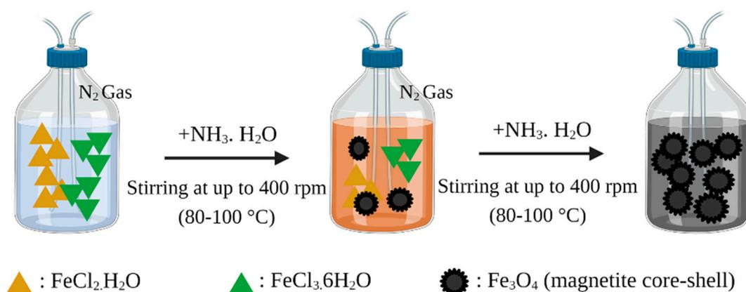
**Figure 2.** Synthesis of magnetic cores: co-precipitation method.
