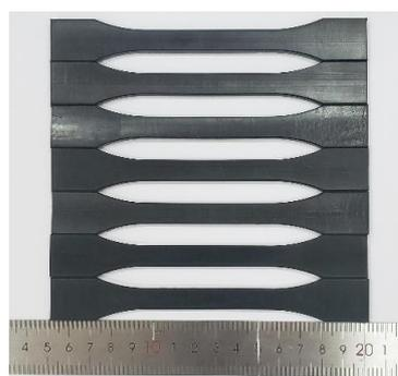
**Figure 1.** Tensile specimens of PE100 pipe material.
