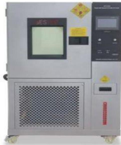
**Figure 2.** Short-term hydrothermal aging setup.
