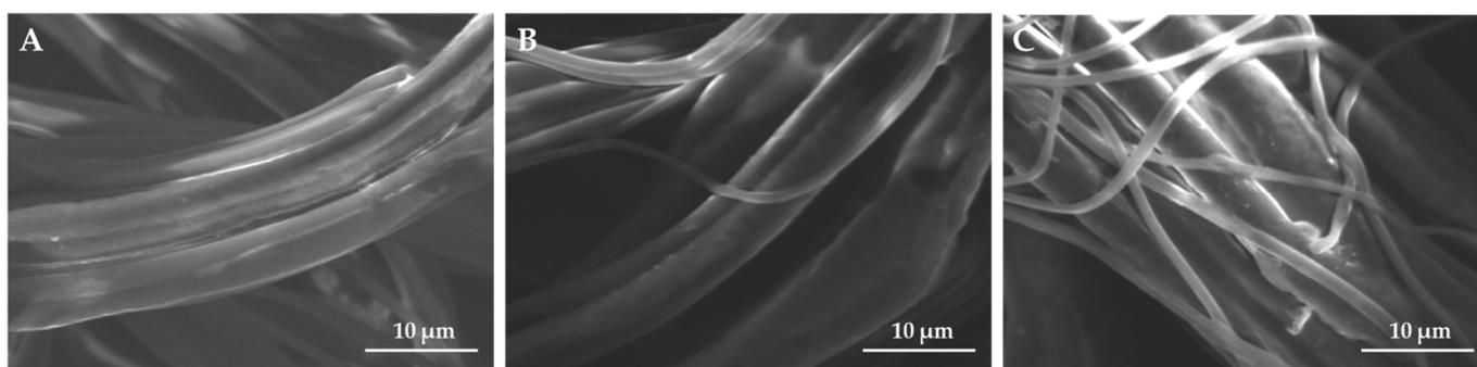
**Figure 7.** FE-SEM characterization of (A) GMA MNWF, (B) IDA-EDC MNWF, and (C) NANA MNWF.
