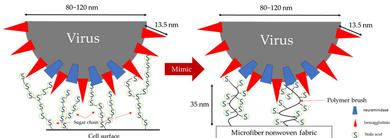
**Scheme 1.** A design concept that mimics the sugar chain cluster effect with sialic acid introduced into the functional microfiber nonwoven fabric.
