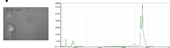
Figure 6. Quantitative evaluation of polyethylene microplastics. (a) Number of detected PE microplastic particles in samples from the 2000 mg/kg group. (b–f) PE microplastics (red circle) detected in lung, duodenum, ileum, serum, and stomach by Raman spectroscopy and wave number of polyethylene microplastics. (g) One plot of wave number of (b–f).
