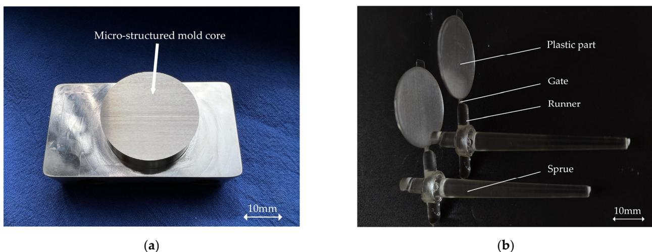
**Figure 1.** Photographs of the micro-structured mold core and parts: (a) insert with microstructure array; (b) injection-molded sample.
