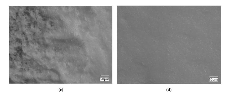
**Figure 12.** Images depicting the different crack growth mechanisms in a PP-1 specimen at  $\Delta K_I$  of 1.09 MPa  $\times$  m<sup>0.5</sup>. Overview image of specimen (**a**) the approximate positions of the three areas from fibrillation (**b**), transition (**c**), and large-scale brittle failure (**d**) are depicted with red rectangles.
