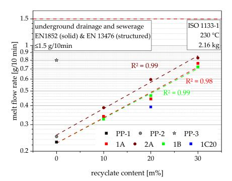
**Figure 1.** Graphical illustration of MFR values of the virgin blending partners PP-1 and PP-2, as well as the virgin injection molding grade PP-3 (as 0 m% recyclate content data points), and the compounds containing 10 m%, 20 m%, and 30 m% rPP-A, rPP-B, and rPO-C, respectively. Linear approximations of the compounding series 1A, 2A, and 1B are plotted as dashed lines, and the respective R<sup>2</sup> values are shown in the matching colors.
