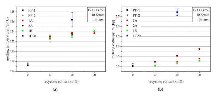
**Figure 6.** DSC results of the virgin blending partners and all compounds in terms of PE melting temperatures (**a**) and PE melting enthalpies (**b**). The vertical bars show the sample standard deviations.
