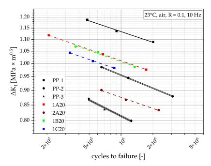
**Figure 10.** Graphical illustration of FCG resistance of the virgin blending partners PP-1 and PP-2, as well as the injection molding benchmark PP-3 and all compounds with 20 m% recyclate content. Initially applied  $\Delta K_I$  as a function of cycles to failure. All lines are linear approximations between three measurement points.
