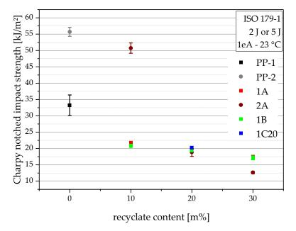
**Figure 9.** Graphical illustration of Charpy notched impact strength of the virgin blending partners PP-1 and PP-2 (as 0 m% recyclate content data points) and all compounds. The vertical bars show the sample standard deviations.
