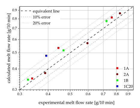
**Figure 2.** Plot of calculated (via Arrhenius mixing rule) vs. experimental MFR values. Most compounds lie within or around the 10% error range. Only 1A20 (0.54 g/10 min calculated vs. 0.44 g/10 min experimental MFR) and 1C20 (0.48 g/10 min calculated vs. 0.39 g/10 min measured MFR) show around 20% error.
