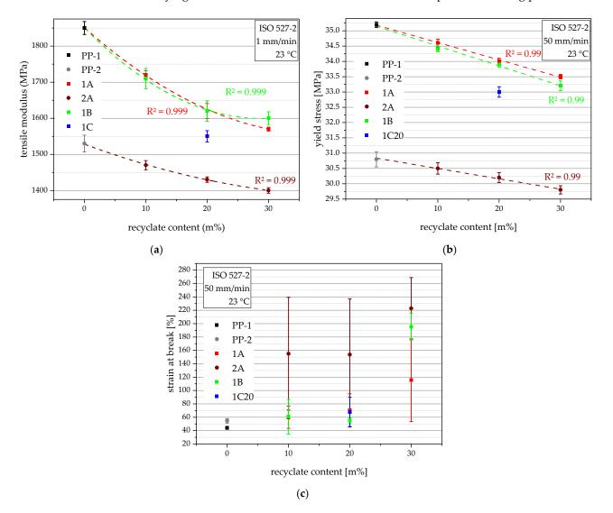
**Figure 8.** Graphical illustration of tensile modulus (**a**), yield stress (**b**), and strain at break values (**c**) of the virgin blending partners PP-1 and PP-2 (as 0 m% recyclate content data points) and all compounds. The vertical bars show the sample standard deviations. Polynomial (**a**) and linear (**b**) approximations depicting the three distinguished compounding series (1A, 2A, 1B) are plotted as dashed lines, and the respective R<sup>2</sup> values are shown in matching colors.
