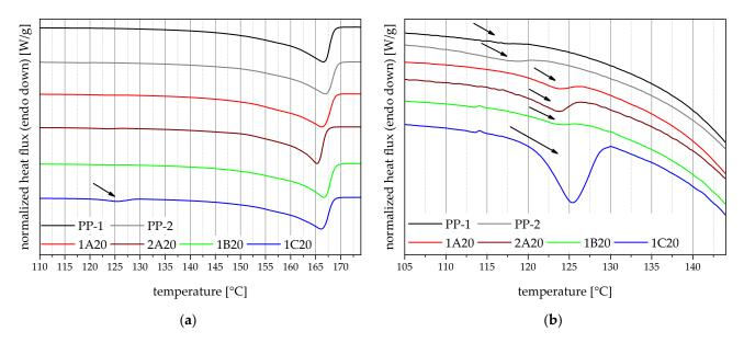
**Figure 4.** Thermograms of the virgin blending partners PP-1 and PP-2, and the four 20 m% recyclate compounds (**a**) and a more detailed look at the PE melting region of these thermograms (**b**). The arrows indicate PE melting peaks.
