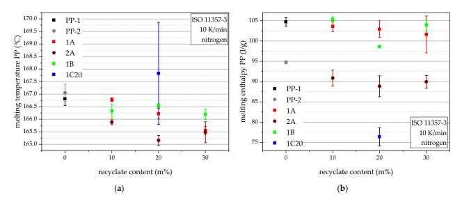
**Figure 5.** DSC results of the virgin blending partners and all compounds in terms of PP melting temperatures (**a**) and PP melting enthalpies (**b**). The vertical bars show the sample standard deviations.
