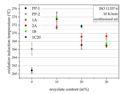
**Figure 7.** Graphical illustration of oxidation induction temperatures of the virgin blending partners PP-1 and PP-2 (as 0 m% recyclate content data points), and all compounds. The vertical bars show the sample standard deviations.
