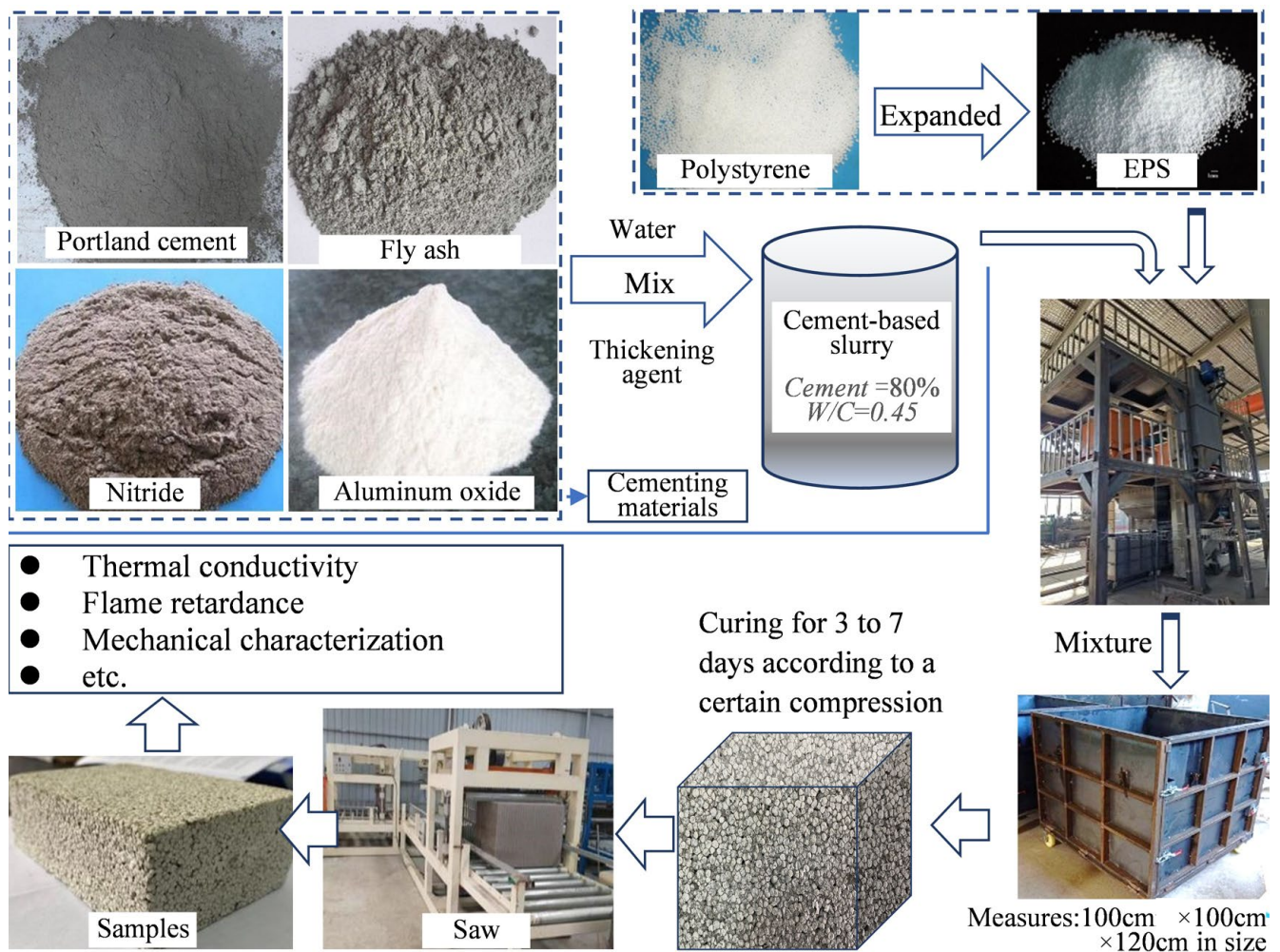
Figure 1. The preparation of CEPS specimen process and test flow diagram.
