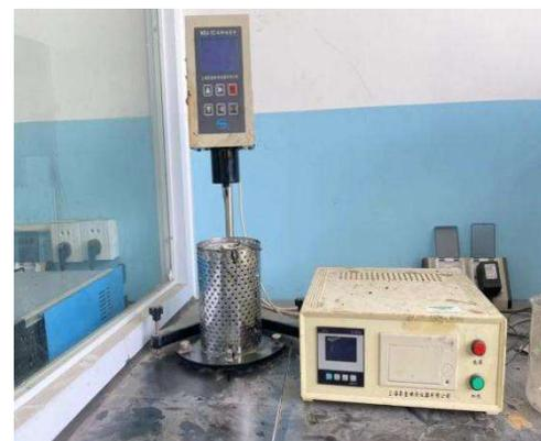
(b) rotary viscometer
