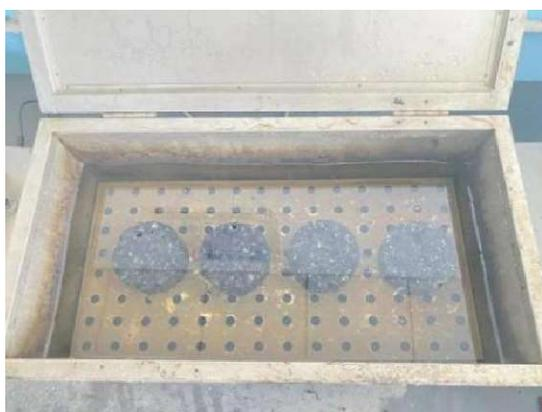
**Figure 4.** Immersed Marshall specimens.
