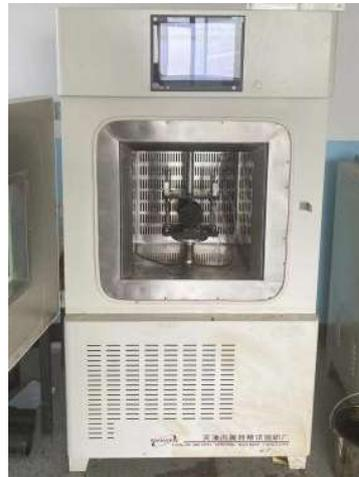
**Figure 5.** Splitting loading instrument of specimens.
