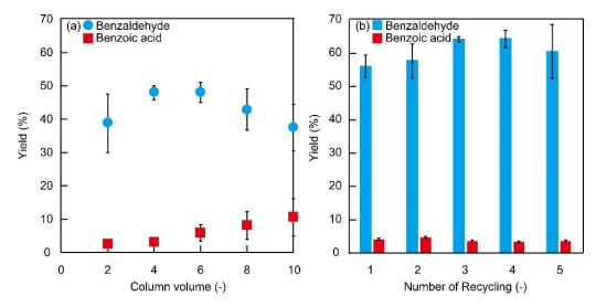
**Figure 6.** (a) Flow oxidation of benzyl alcohol by Monolith—1 at a residence time of 4 min. (b) Recycling test for flow oxidation of benzyl alcohol by Monolith—1 at a residence time of 4 min, and the yield of 4-column volume is shown.
