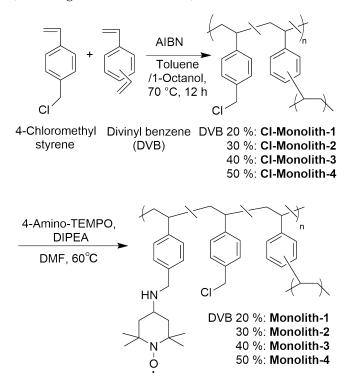
Figure 2. Preparation of Monolith (4-amino-TEMPO-immobilized monolith) with Cl-Monolith.
