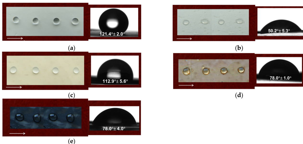
Figure 5. Digital images of water droplets (10 \mu L) deposited on the surfaces of fibrous mats from (a) PLA, (b) Ch/PLA, (c) Ch-8Q/PLA, (d) \text{Cu}^{2+} complex of Ch-8Q/PLA and (e) \text{Fe}^{3+} complex of Ch-8Q/PLA. The direction of the collector rotation is indicated by an arrow.
