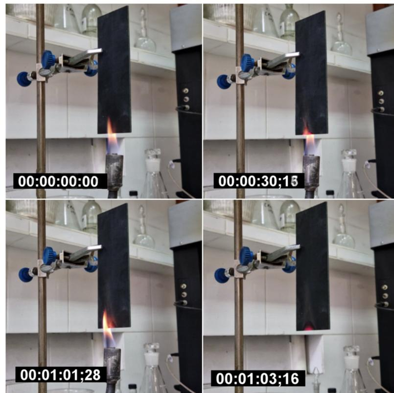
Figure 10. GFRP burning at 900 for 60 s.
