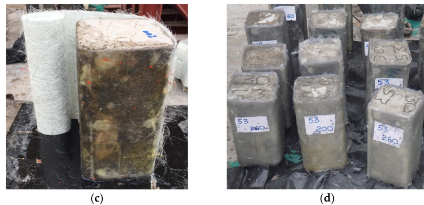
Figure 4. (a) Steel molds, (b) application of resin using a roller, (c) FCSM wrapping in progress, and (d) strengthened specimens.
