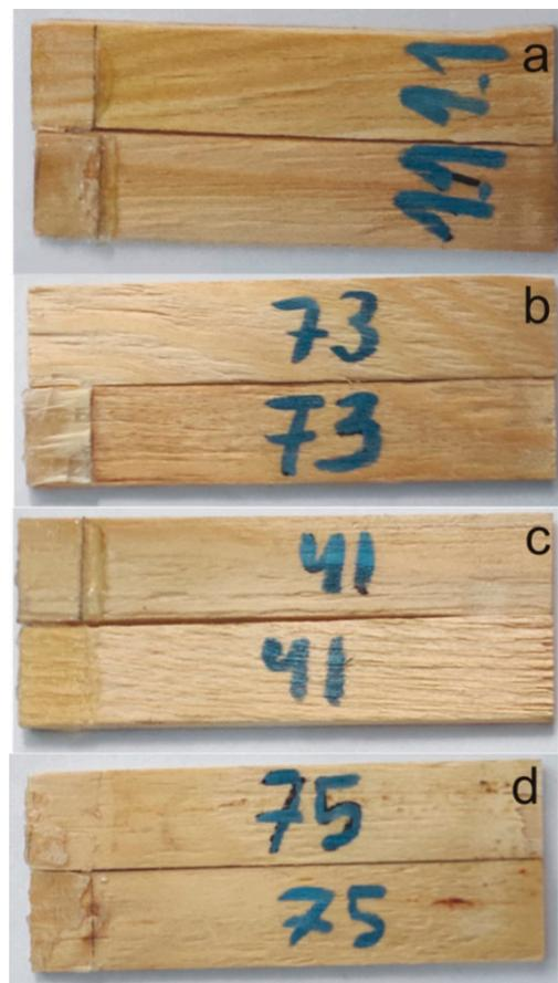
**Figure 6.** Failure modes observed in the tested specimens: (a)—adhesive at the binder/wood interface, (b)—cohesive in wood, (c)—cohesive in PHU layer, and (d)—mixed.
